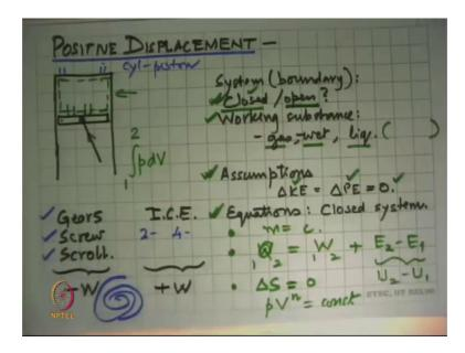
First thing that I will do that is what I have listed here as positive displacement devices and for positive displacement, we mean that once you have a substance in that take an inside the device, no matter what the outlet condition, when you operated, it will push it out. There is no way that it will just stay inside.
