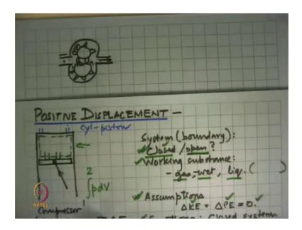
So, there; this is the gear, and this is in mesh with another gear and the space around this is very tightly controlled, there are very small clearance between them. One of this is connected to the inlet, this is connected to the discharge. And what it does is its track this fluid which was trapped here, it will be carried forward and physically pushed into this thing, so that is how you can have two gears in mesh doing the job of a compressor or a job of a pump.
