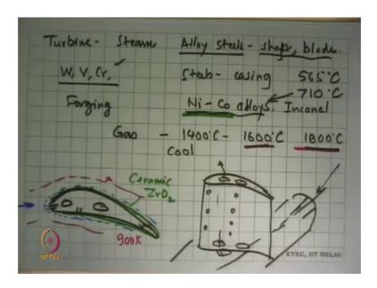
We come to turbine now; first we have the steam turbine. And these are alloy steels, alloy steel for the shaft, and the rotating parts the shaft, blades, and rotating parts. And types of steels for casing the stationary parts, these the real high tech part or these rotating part, because they are not just at high temperature, but they are also rotating, they are transmitting torque. And it has lot of blades on it, they would have also be (Refer Time: 06:16). So, these are alloy steels.
