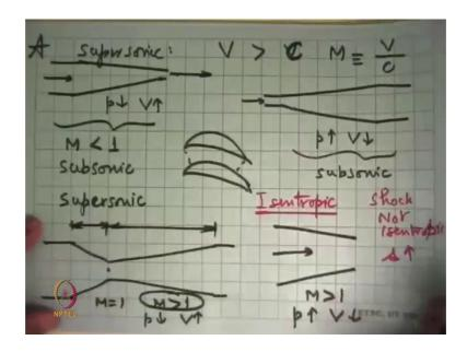
The next question was what about supersonic flow in a nozzle right, so this is what it is? When we say supersonic flow, what we mean is that the local velocity is greater than the local speed of sound or C. I am using the word local, because if you have say a nozzle as the flow goes through it, its temperature is changing. So, when the temperature at different locations is different, so local speed of sound is also there.
