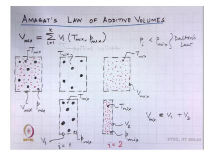
We now go to the second law, which is Amagat's law of additive volumes. Simply put it says that V mix is the summation of V i provided the component occupy is at the same temperature, and the same pressure as the mixture. So, here is what it means that is this is the system. And we have two components there, one is this one, and the others are here.
