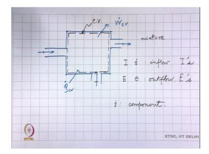
Now, we come to a conservation equations for gas mixtures for an open system. So, what we are doing here basically is like before we say that there is a system in to which there are different inflows and outflows across which, there could be heat transfer, and work transfer. And for that we define the control volume, which is say all this part of the substance in this control volume. The only difference is that these states here all of them would have a mixture.
