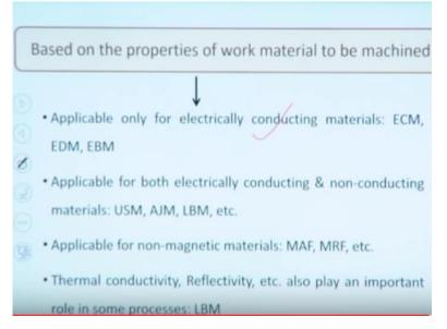
So this classification of advance machining process is based on this properties of this orifice materials of machine okay. So applicable only for electrical conducting materials like ECM, EDM, and electron beam machining process, applicable for both electrical conducting and non-conducting material okay. So these ultrasonic machining, AJM abrasive jet machining and laser beam machining it can be machined for both electrical conducting and non-conducting material.
