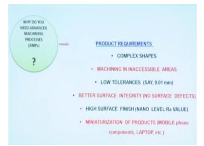
So why we need advanced machining processes? Here product requirements are complex shapes machining of inaccessible areas. Suppose some inaccessible areas are there, there we have to do the machining operations. So the only possible solution is that advanced machining process okay. So suppose we have to gain the very low tolerances say 0.1 mm so we cannot achieve very low tolerances in case of conventional machining process.
