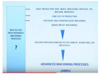
Showing in high metal removal rate also. So high production rate while processing difficult machine materials, low cost of production and then precision and ultraprecision machining, nano-meter machining will lead to the requirement of material removal in the form of atoms and molecules okay. So now the solution is that advanced machining process.
