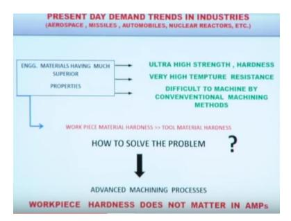
So engineering materials having much superior properties okay as high ultra high strength, ultra high hardness. So these materials are high strength temperature resistance material okay. So one of the materials of this high strength temperature resistance material is used in turbine blades okay where minimum temperature is attained as 1100 degree centigrade okay.
