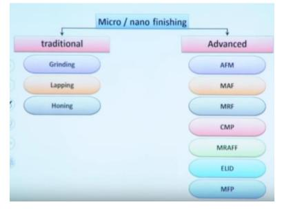
So nano finishing also traditional nano finishing process like grinding, lapping, honing operations are there and advance nano finishing process like AFM abrasive flow machining, magnetic abrasive finishing, magnetorheological finishing, chemomechanical polishing, magnetorheological abrasive flow finishing, electrolyte in-process dressing. So these are the advance type and then magnetic float polishing.
