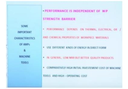
So these kind of thousands of examples are there okay. So this abrasive machining processes performance is independent of the orifice material strength okay. So there is no strength barrier is there. Performance is depends on the thermal or electrical or chemical properties of the orifice material. So material hardness does not matter.
