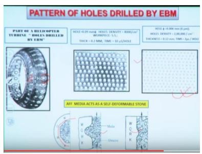
So patterns of holes are generated. So this is the part of a helicopter turbine. You can see at the surface of this turbine different types of cross-sections of holes are generated. So these cross-sections and these cross-sections are entirely different. So this kind of thousands of holes are actually generated at the surface of this turbine.
