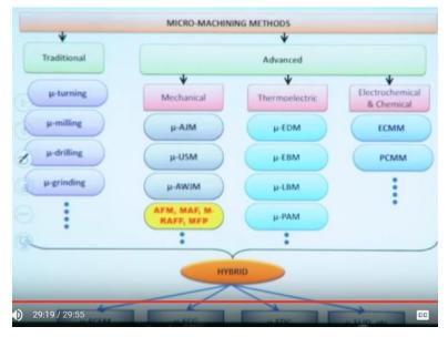
So micro-machining methods different micro-machining methods, traditional micro-machining which are used like micro-turning, micro-milling, micro-drilling, micro-grinding okay. So micro-machining advance type of micro-machining processes also like mechanical, micro AJM, micro ultrasonic, micro abrasive water jet machining, abrasive flow finishing, magnetic abrasive finishing, magnetorheological abrasive flow finishing, magnetic flow polishing okay.
