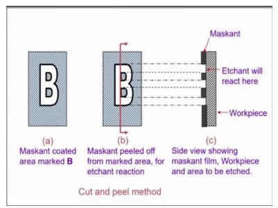
So this is the workpiece here, maskant coated already. So if you see the cross section of this maskant, if you take a cross section here along this line you can see so this is the workpiece material, here this maskant layer and this is the exposed area where we need the machining to be
