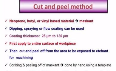
✓ Accuracy obtained → 130 µm to 750 µm depending upon size & type of component being produced
