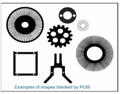
So this kind of complicated surfaces can be generated by using the photochemical method. This complicated details so these kind of complicated details can be generated by photochemical machining process.
