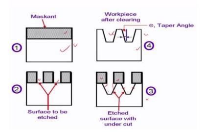
So this is the schematic view of chemical machining process. Here this is the workpiece. On this workpiece this chemically resistant material that is the maskant actually used, a maskant layer is used, deposited on the workpiece surface and this is the second one. After that this maskant from some selective area this maskant is actually scrapped or removed from some selective area.
