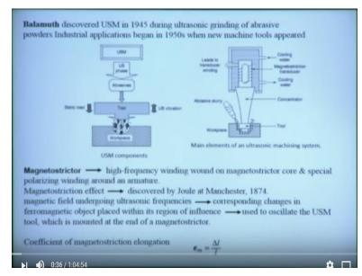
As I told that it was ultrasonic machining process was discovered by Balamuth in the year of 1945 during ultrasonic grinding of abrasive powders, industrial application begins in 1950 when new machine tools appear okay. So we have discussed that there are 2 types of magnetostriction transducers are there, one is magnetostrictive type, another one is the piezoelectric type okay, 2 transducers are there.
