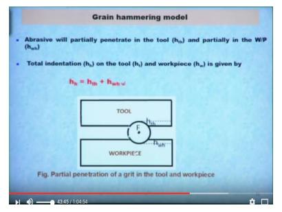
So again so this abrasive will partially penetrate in the tool as well as into the workpiece so total depth of penetration is equal to the hammering model indentation if the indentation due to the into the tool and indentation into the workpiece.
