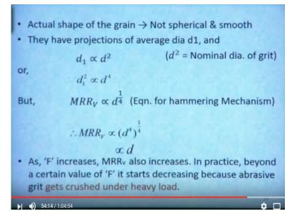
So actual shape of this grain it is not a spherical, it is not a spherical it is random in size. The abrasive particles are random in size but we have considered this one as spherical and smooth. So it is not at all spherical and smooth. So they have a projections of average diameter of this d1
