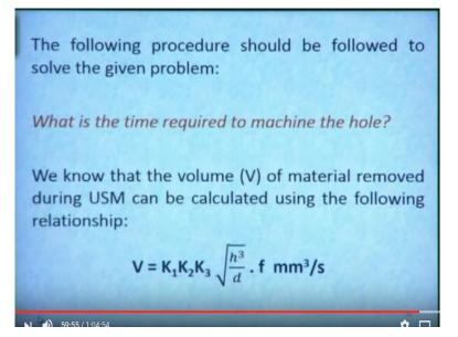
So there are different steps. The following procedure should be followed to solve the given problem. So what is the time equal for machining the hole of 6 millimeter diameter okay. So now volume of material removed we know this equation 1. So this is equal to K1 K2 and K3 root over H cube by d. So here unknown is the H. So H we have to calculate first by hammering model as well as by throwing model okay.
