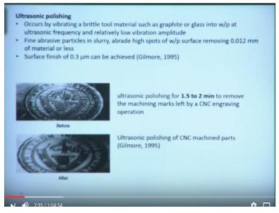
So ultrasonic polishing. So ultrasonic machining process, the same process can be used for polishing purpose also. So in this case even the amplitude of vibration is very less okay. So
