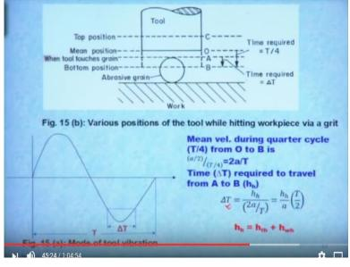
So what is the mean velocity between the quarter cycle T/4? So from here to here it is the T/4. What is the velocity here? At this point this tool is actually going half of means it is going to the amplitude amount okay so this is a/2 amount, it is moving. So amplitude of vibration is a/2 here okay. So what is the velocity here? Velocity we can calculate this a/2 divided by T/4 okay. So this with this time T/4 it is moving a/2 amount of depth means a/2 amount of depth okay. So so
