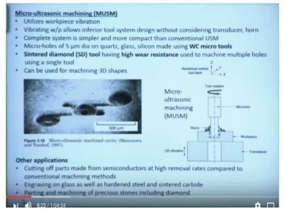
So another application is the micro-ultrasonic machining okay. So in this case your tool is very small okay. So utilizes workpiece vibration, vibrating workpiece okay. So instead of giving vibration to this tool here vibration is given to the workpiece itself okay. So vibrating workpiece allows inferior tool system design without considering transducer, horn okay. So micro-holes of 5 micron diameter on quartz, glass, silicon made using tungsten carbide micro tools.
