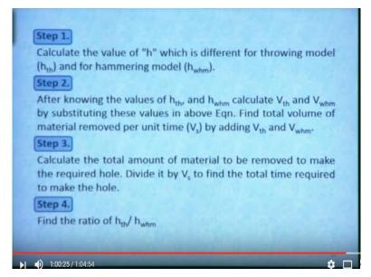
This step 1 this calculate the value of h which is different for throwing model and hammering model. So after knowing the values of this h for throwing and hammering model calculate the volume of material removed by throwing model by this earlier equation and volume of material removed by the hammering model by substituting these values of this h into the equation last in the last equation okay. So now we can find out the total volume.
