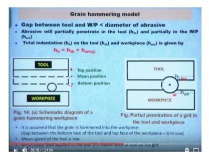
So this is the okay. So here this is the tool here tool at the top position here. Now it will come to the mean position. After that it will come to the bottom position and this bottom position it will hit the abrasive particles because here gap is less than the gap between this tool and the workpiece top surface of the tool and the workpiece surface okay.
