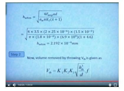
So by hammering model it is 4 average a average to the vibration is the diameter of this abrasive particle, sigma w is the hardness of this workpiece material then K2 is the constant lamda is the ratio by throwing model by indentation by throwing model by hammering model okay. So here we known all these values. After that we shall get this we can get this on this indentation by the hammering model here.
