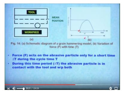
So force acting on the abrasive particle only for a short time del T okay. Now you can see so from this top position it will come to the mean position after that it will come to the bottom position. So while coming to this bottom position it will touch at this point to the, this tool will touch in contact with the abrasive and then abrasive is in contact with the workpiece okay. So at this point only there is a contact between this tool, abrasive, and workpiece starts.
