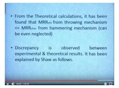
So from the theoretical calculation it has been found that MRR by throwing model from the throwing mechanism is very very less than this hammering mechanism okay. So material removal rate from this throwing mechanism is very less than the hammering model okay. So we can neglect that material removal rate from the throwing model. So discrepancy is observed between the experimental and theoretical results and it has been explained by Shah as follows okay.
