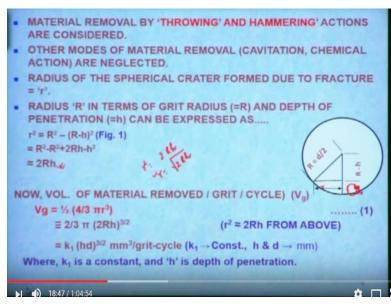
Okay so material removal by throwing. There are 2 types of models are there. One is the throwing model, another one is the hammering model okay. So other methods of other
