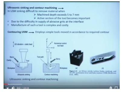
So there are another applications by this ultrasonic machining process. So this is called ultrasonic sinking and contouring machine okay. So this is the first case when we give this ultrasonic sinking operation okay so here ultrasonic vibration and we are giving some static field to this tool.okay. So now this is the shape of this tool okay so we do not we want to make same shape of this tool into the workpiece surface. So it is called actually ultrasonic sinking operation.
