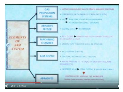
So what are the different elements of abrasive jet machining. So first one is the gas propulsion system. Second is the abrasive feeder system. Third one is the machining chamber and then fourth one is the abrasive nozzle and fifth component of this abrasive jet machining process is abrasives okay so these are the different components.
