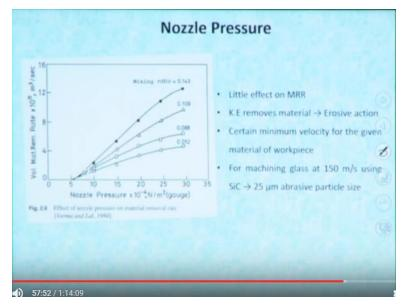
So nozzle pressure, so nozzle pressure has a little effect on material removal rate. So this kinetic energy removes the material so because of this kinetic energy this erosion takes place on to the workpiece surface. Certain minimum velocity is required. So this is called the critical velocity. So this is the critical pressure. Certain minimum critical pressure is required.
