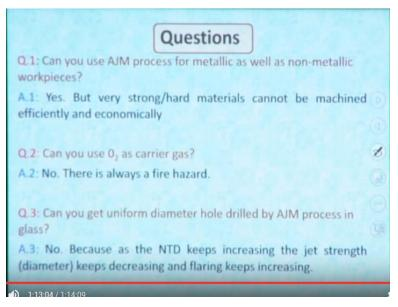
Question, can we use abrasive jet machining process for metallic as well as non-metallic workpiece, yes. So it can be used for metallic and non-metallic but this workpiece should be strong and hard materials. So workpiece should be very hard.
