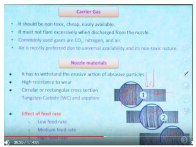
So carrier gas, so what are the properties of this carrier gas. They should be nontoxic, cheap, and easily available. It must not flare excessively when discharged from the nozzle. So commonly
