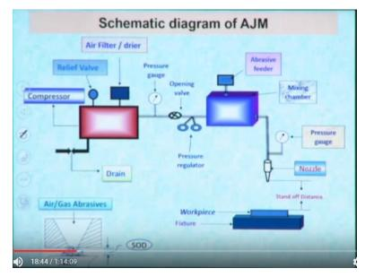
So now we shall discuss what are the different components of abrasive jet machining okay, so experimental setup of abrasive jet machining process okay. So now this is the schematic diagram of this process. Here we can see that so here we need a compressor. So why we need a compressor because to generate the high velocity jet we need a very means we need a compressed air okay. So for making this for generating this compressed air okay we need a compressor.
