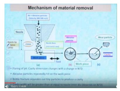
So again it is shown in this figure. So it this is the nozzle here. So the abrasive particles from air is coming with a very high velocity. So this distance nozzle tip nozzle diameter is 0.3 to 0.5 mm. This stand of distance is 1 mm here okay. So this workpiece actually this nozzle actually it is fixed to the machine or this workpiece is actually attached to a CNC table okay.
