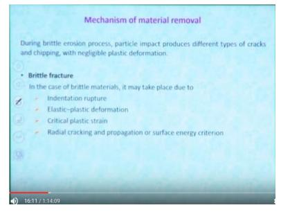
So there are 2 mechanisms I told that on this it is useful for hard and brittle material. So because of this in brittle material these are the mechanism occurs, indentation rupture, elastic-plastic deformation, critical plastic strain, radial cracking and propagation of surface energy criteria. So these are the things during brittle erosion process particle impact produces different types of gas and chipping with negligible plastic deformation.
