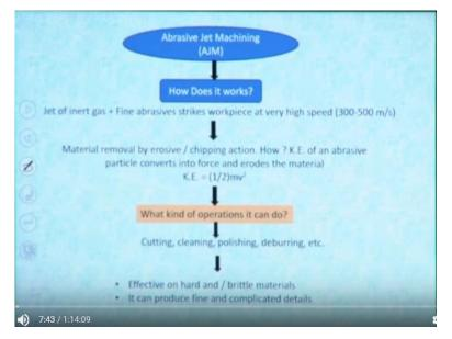
So now what is the working principle of abrasive jet machining process. In abrasive jet machining process high velocity abrasives in a media of air it is impinging on the workpiece surface okay so when it is impacting on the workpiece surface it will make a brittle fracture or it will generate a small crater into the workpiece surface.
