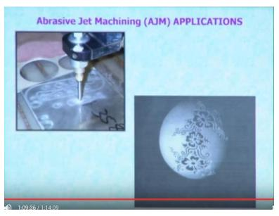
There are 3 applications you can see using this abrasive jet nozzle this kind of complicated details you can generate into the so these complicated details also you can generate into the workpiece. So this kind of complicated details can be generated into the workpiece. So here is the example of abrasive jet machining. So these kind of design can be generated on a egg shell okay. So on an egg shell actually these kind of design is generated.
