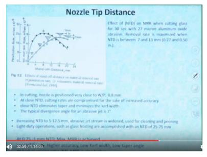
So now this is the effect of nozzle tip distance okay. So on penetration rate, so penetration rate already we have discussed. Penetration rate while we are doing the impacting by this abrasive jet machining. So penetration means this depth of indentation will increase okay so with time. So this is the penetration rate. So it is mm/sec. So what is the depth what is the depth increasing depth with time so that is called the penetration rate.
