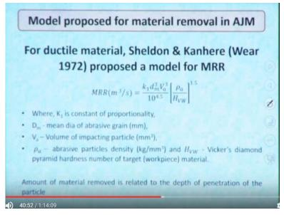
So for ductile material also Sheldon and Kanhere they proposed a model for calculating material removal rate for ductile material. So it is published in Wear in 1972. So here material removal rate it is it is proposed in this this is millimeter cube it should be millimeter cube. So this material removal rate is millimeter cube per second. So equal to k1 d suffix m cube then V suffix a cube by 10 to the power 4.5 multiplied by rho a by Hvw.
