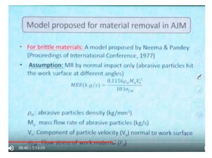
Now we shall discuss some models of material removal mechanism or abrasive jet machining process. So there are 2 models we shall discuss. So first one is the for brittle materials. So this one is this model was actually proposed by Neema and Pandey in 1977 and it was actually published in Proceedings of International Conference okay.
