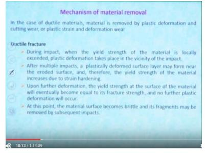
Upon further deformation the yield strength at the surface of the material will eventually become equal to its fracture strength and no further plastic deformation will occur. So at this point material surface becomes brittle and its fragments may be removed by subsequent impacts.
