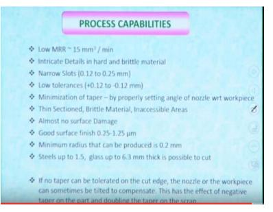
Okay, process capabilities. So process capabilities it has a very less material removal rate 15 millimeter cube per minute. So low material removal rate. So intricate details in hard and brittle materials. So it can generate intricate details on hard and brittle materials because abrasive particles need not touch means tool does not touch the workpiece surface like in conventional cutting or milling operation while tool detect it as the workpiece surface.
