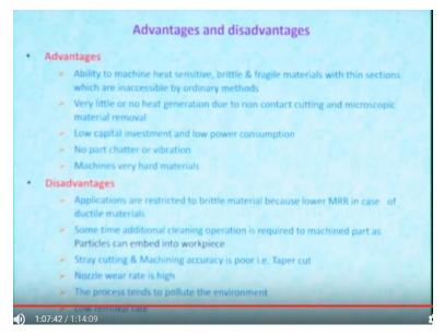
So there are some advantages and disadvantages of this process. Advantages are machine is heat sensitive. So heat does not means heat is not generated. Whatever heat is generated it is taken away by the carrier gas. Very little or no heat generation to non-contact cutting and microscopic material removal very small small material removal is there.
