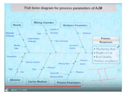
So now we have to do the parametric analysis. What are the different first we have to find out what are the different parameters are there and then we have to select what is the effect of parameters on process performance. So this is the fish bone diagram for this process parameters for different process parameters in abrasive jet machining process.
