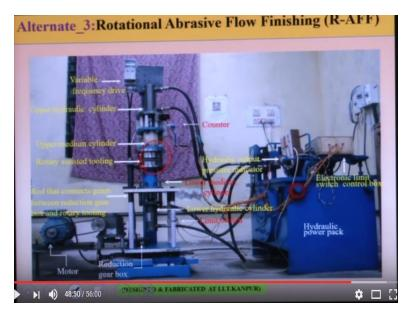
Another thing is that actually you can rotate the media here by an external means. So this is called rotational abrasive flow finishing process. You can rotate this media itself. So here whatever workpiece fixture workpiece tool is there that can be rotated by an external means okay.
