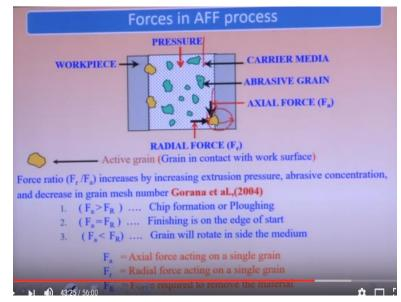
So what are the different forces are there in abrasive flow finishing process? So you can see that this media is flowing through this cylinder okay. So these are the abrasive particles are there. These abrasive particles it is indented into the workpiece surface and this indented workpiece it is moving towards the because of this axial force these indented abrasive particles are doing surface undulations from the workpiece surface okay.
