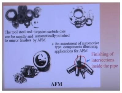
So I told initially that this kind of intersections of this holes here so many holes are actually pipes are actually connected here. Here you can see it is not a smooth at the intersection of this tools. Thus intersection of this tools can be polished by the abrasive flow finishing process, this kind of small components can be polished by AFM process.
