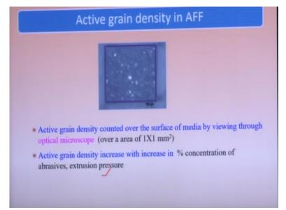
So if active grain density is less we have to increase the concentration of this abrasive particles so that this active grain density can be increased. So it can increase, this active grain density can be increased with the increase in the percentage concentration of the abrasive particles. Also increasing the extrusion pressure also your active grain density can be increased okay.
