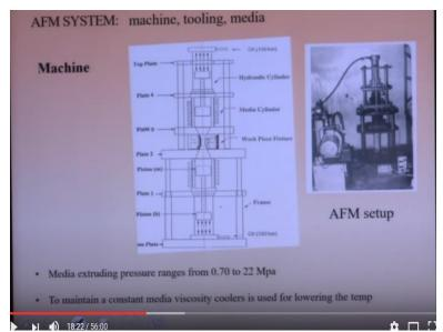
So in this setup you can see the machine, tooling, and media here okay. So media pressure here they have considered 0.7 to 22 MPa here. So to maintain the constant media viscosity coolers are used for lowering the temperature. So this media it its property actually dependent on the
