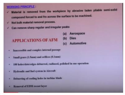
So what is the working principle, working principle of abrasive flow finishing process? Material is removed from the workpiece surface by abrasive laden pliable semi-solid compound forced to and fro across the surface to be machined. It is not a bulk material removal process. It is a selective material removal process. Can remove sharp regular, irregular peaks.
