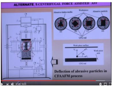
So how to enhance the performance of this abrasive flow finishing process? To enhance the different researchers actually they developed different process to enhance the performance of this abrasive flow finishing process. So this is actually centrifugal assisted abrasive flow finishing process here okay. So here you can see this is the workpiece here. At this workpiece at the center actually there is a centrifugal rod. So here you can see cross-section of this workpiece here.
