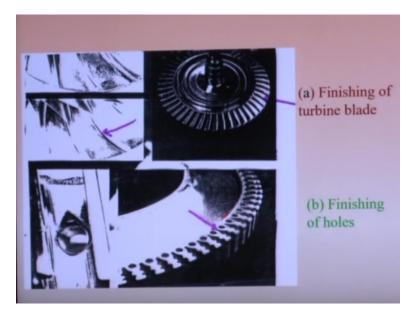
So this kind of turbine blades can be polished by this AFM media. This kind of small holes can be polished by this finishing holes can be polished by AFM media.
