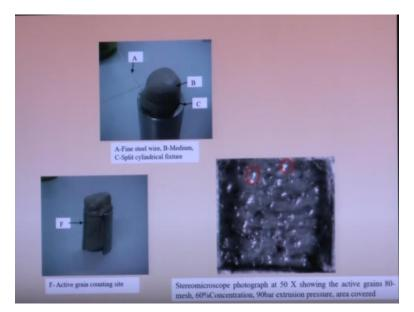
So here you can see this is the media here okay. So this media you can see under microscope. So these are the white spots. This white spots actually these are the abrasive particles okay. It is shown under 50 X optical microscope okay.
