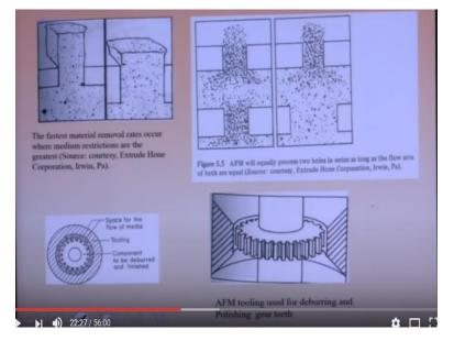
So now you can see this restrictions, so here this small cross-section, here it is the bigger crosssection okay. So we can expect that means higher material removal rate will be here than this material removal rate here okay. So here also lesser restriction here means maximum restrictions are here lesser restrictions are there.
