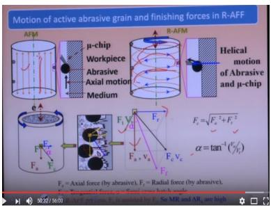
You can see what are the forces are there. This radial force is there because you are flowing you are giving reciprocal motion radial force is there and this axial force is there and this tangential force or coriolis tangential or coriolis force is added here. This coriolis force actually this coriolis force it is generated because of this rotation of this media okay. So this tangential force will helps in cutting the surface undulations.
