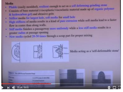
So any kind of complex surfaces can be polished by using this process, abrasive flow machining process. So another thing is that media. So another component of this abrasive flow machining process is the media. So this media is a pliable, easily moulded, it can be moulded easily, it can take the shape of the workpiece surface resilient enough to act as a self-deforming grinding stone. So grinding stone you see you know this grinding stone is used in grinding operation.
