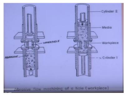
So this is the working this is the schematic diagram of abrasive flow finishing operation. Here you can see there are this is one piston, this is another piston, 2 pistons are there. So this is the 2 piston. This is called top piston. This is the bottom piston, bottom media piston, and in between you can see this is the media. So this is the viscoelastic polymeric media okay. So this viscoelastic media it is given to and fro motion.
