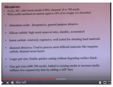
When media is machined an amount of 10% of its weight. Suppose you are doing the machining and your or initially your media weight of this media is suppose 1 kg. Now after machining whatever debris particles are there that will also come into the media okay. So after machining for many components you will see this media weight will increase because whatever debris particles that are also mixing with the media.
