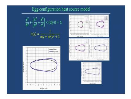
There is another type of the heat source that is called development happens that is called egg configuration heat source model. Here you can see the equation is basically we use the ellipsoidal when you try to develop the illustrator heat responded we use this equation, but if we use just multiplying the factor t y any functional form we can modify the equation a different way.
