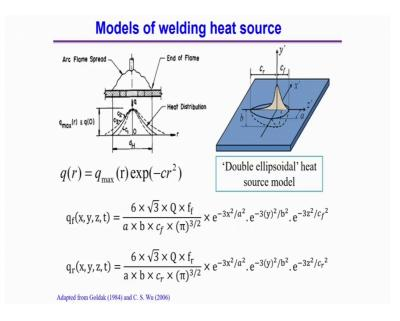
Now, we start from the models of the heat source were just look into that dicks type of heat source here you can see that top figure it is a representation of the art normally we can see the end of the flame happens over a certain boundary that with respect to the center and this is this follows generally typical Gaussian distribution. Now, this heat distribution in mathematical representatives of the heat distribution we can use this
