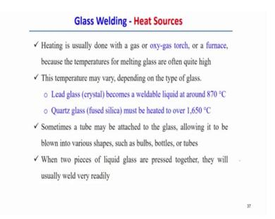
So, normally welding with gas or oxy gas torch hot oxy gas torch or using a furnace the these are the typical source of the glass and we it is easily to locally applied in certain part of the glass and then melting of the glass happens and finally, joined between these two components. But, typically the glass the melting of the glass is often quite hard quite high therefore; the furnace is one of the choices of heating the act as a heat source for the welding of the glass materials.
