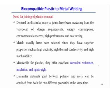
Now, there is a nowadays there is a huge application of the plastic components specifically biocompatible plastic components with the combination of the metallic materials. We can find out this some requirement in specifically in the medical instrument or medical industry. So, therefore, joining of the these two components plastic to the metal is having some significance.
