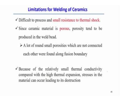
So, it is very difficult to process the ceramic materials, because most of the case we can find out the ceramic is also in brittle in nature and small resistance to the thermal shock load. So, in that sense it is difficult to process.
