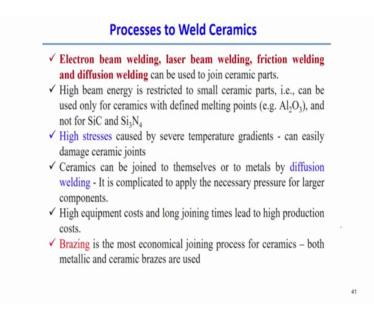
Now, what are the typical joining or welding techniques for the ceramic materials. So, here you can see that; electron beam welding, laser beam welding, friction beam welding and the diffusion welding these are the main processing main processing techniques for the for the welding of the ceramics. So, high beam energy actually restrict application of the high beam energy is basically restricted to the small components of the ceramics.
