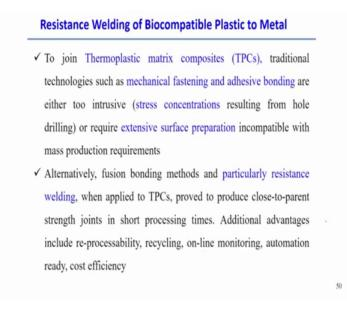
So, of course, if we look into resistance that TPC, that is the polymeric material and joining process such mechanical fastening and adhesive we can use it, but point is that, here if we use the mechanical processing, we can find out the stress concentration due to the hole drilling that is a one things and there is a extensive surface preparation also required, so that actually incompatible for the mass production requirements.
