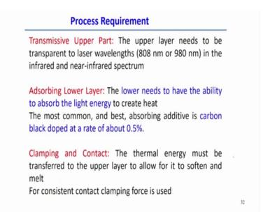
So, if you look into further the process requirement for the laser transmission welding is
