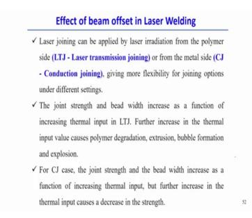
So, here we can see that already, we have discussed about the laser transmission welding or laser transmission joining in this case the polymeric materials normally we can keep on the as a transparent material on the upper side and lower side, if we put the metallic material, so then therefore, at the interface; so heat will be release on the metallic material and then we can join by the laser transmission welding specifically easy to do that in joining between metal and the plastic.
