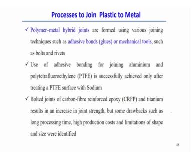
But there are several methodologies also developed for joining the plastic two metals; one is the this polymer metal hybrid joints are found using the various joining techniques simply use some adhesive bonds, simply using some glue or some mechanical tools, that is the most convenient way to join between these two components.
