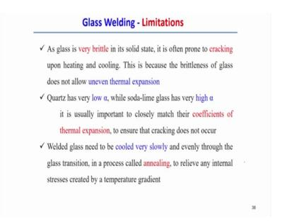
So, because cracking since glass is very brittle material. So, there is a hardly it is very difficult to absorb the uneven thermal expansion during the heating or during the cooling phase. So, there is highly chance to form of the cracking phenomena and during the processing of the glass specifically; when you try to do the welding of the glass.
