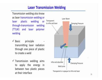
So, we can keep the upper side the transparent material through which, laser beam can passes. And at the bottom side we can put the other different carrier of plastic material such that at the interface there may be the heat generation, such that the two components can be joined here.
