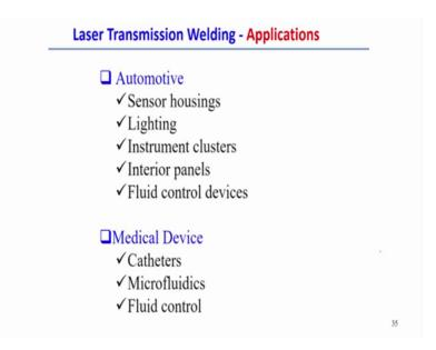
But, if you look into that other application area of laser transmission welding here see the several applications. So, automotive that sensor housing, lighting, instrument clusters, interior panels, fluid control devices, all this in or automotive sector we can find out the application of the laser transmission welding for this material for this area.
