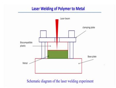
So, here you can see that joining schematic diagram in the laser welding experiment, that is the welding between the polymer to metal. It is a similar configuration to the laser transmission welding, if you see the which is biocompatible plastic normally we can put in the upper side, and in the lower side it is a biocompatible plastic and the lower side is the metal such that laser beam process through the transparent biocompatible metal plastic and heat is generally less at the interface.
