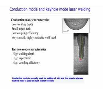
Both the cases that stainless steel has been joined using the laser welding processes.
