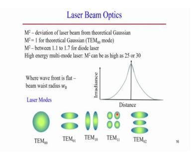
If you see the other critical term which is the laser beam optics that is the m square m square is the represents one parameter that deviation of the laser beam from the
