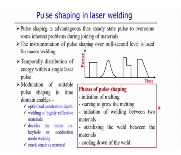
So, pulse shaping is advantageous in the sense that steady state pulse to overcome the some inherent problem during the joining of the material the shaping pulse shaping of the millisecond pulse basically is estimated based on the practical application of this; that means, simply pulse shaping.
