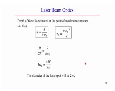
Now, depth of focus is estimated at the point of maximum curvature; that means, at Z equal to Z R. So, in this case theta simply estimated in terms of the laser wavelength lambda by pi into w 0 and from here theta equal to this and plus another equals theta equal to D by two twice f from these two approximation we can find out the relation D by 2 f equal to lambda by pi w 0.
