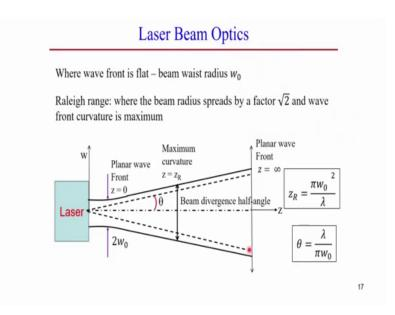
And it is the diverging, but laser source is at actually not is a point source its a sub diameter that planar wave front can be created at a at a specific diameter size that is two w omega w 0 and that is the that is called the where the beam wave front is flat that is called that beam waist radius equal to w 0.
