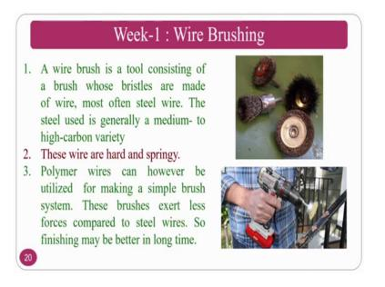
So, wire brushing basically uses metallic which is hard and springy. Some of the applications for fine finishing applications and other things people can go for polymer based also.
