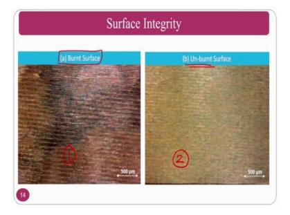
That is why you have to see the surface this is a burnt surface in a grinding process 1 is burnt surface and 2 is unburnt surface if you are going to put one then your life of the component may come down compared to 2. That is why you should always choose better surface roughness as well as surface morphology and surface morphology and surface roughness both are approximately similar and surface metallurgy is different. (Refer Slide Time: 16:22)
