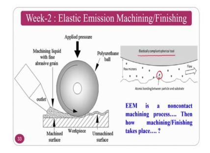
So, you are rotating a polyurethane ball and the abrasive particles and slurry is coming in contact and there is no contact between the elastically complaints spherical tool as well as the workpiece surface. Only thing is that the particles that are going to use in elastic emission machining are finishing is going to come in contact with the workpiece material. In that circumstances this particular process is called noncontact finishing process. So, then how the material removal takes place ok.
