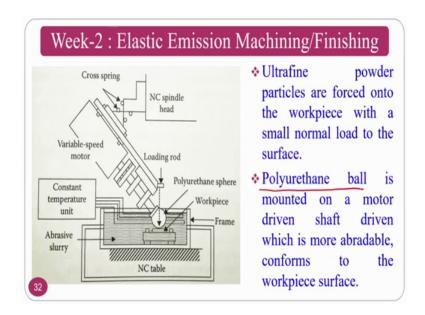
So, elastic emission machining process where you can see a ultrafine powder particles are forced into workpiece where there is a polyurethane ball is there mounted on a motor and you are going to drive it and what you can see here is.
