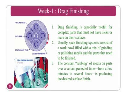
And here the component can be finished locally there all the components are placed in a bowl and rotated. So, it is a global and this is global plus local.
