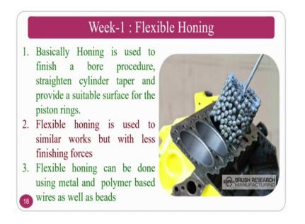
Now, we will move on to another thing flexible honing process. Basically honing is used to finish a bore and other things and in a flexible honing process instead of your honing sticks you will come across with a beads ok. So, these beads may be prepared with the metallic or it can also be prepared with a polymer. At the same time some of the agencies can also fabricate these with both ok.
