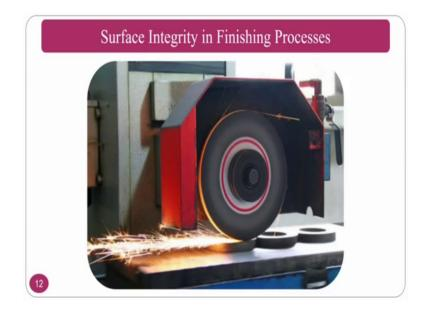
First conventional finishing process whenever you see what you are going to get into your mind is the grinding process. So, grinding process if you see lot of spark is coming here because of the friction that is generated between the grinding wheel as well as the work piece because of this the temperature goes enormously high ok.
