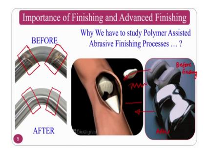
And you can see what is the importance of finishing as this is the before finishing you can clearly see here how the weld joints are looking like ok. So, after finishing you can clearly see how these are disappeared. If you are going to use the same thing in a practical application without finishing then your performance will enormously go bad ok. That is why you require finishing in a great way the same thing if you can see for a
