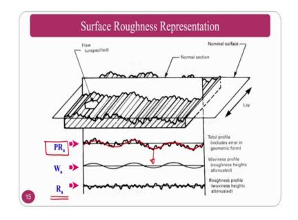
So, once you know the surface metallurgy is fine and you have to go for surface roughness representation. The surface roughness you can represent in terms of three profiles basically what we always check is surface roughness, but some of the people will always represent in a profile roughness as well as waviness. And other things the profile roughness PR a which you are seeing here you can divide into waviness as well as roughness.
