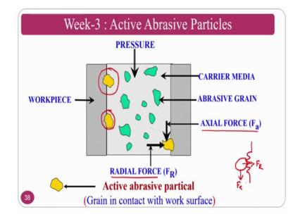
As I said what is the difference between active abrasive particle and inactive abrasive particle. Whenever you are reciprocating the medium by exerting some pressure what will happen those particles that come in contact with respect to workpiece are nothing, but active abrasive particles ok. And what are the pressures that are involved here is radial pressure as well as the forces that are involved in this particular process is axial force as well as radial force.
