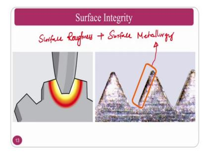
So, the basic problem comes is whenever you are grinding wheel is rotating or a form grinding wheel is rotating at a high speed temperature generates. Because of the temperature what will happen is there will be burning and there will be surface roughness. That is why surface integrity means the surface roughness one is surface roughness plus surface metallurgy ok.
