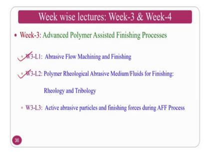
So, week 3 we are going to see the advanced polymer assisted finishing process where you can see the abrasive flow finishing process and abrasive flow machining process why it is called abrasive flow machining as well as why it is called as abrasive flow finishing process. Then polymer rheological abrasive medium and its rheology then we will see what is active abrasive particles and how this finishing process will help in removing the material.
