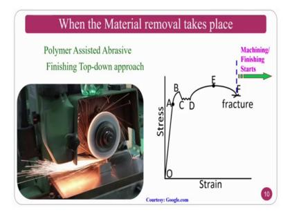
That is why as you know the material removal processes are subtractive manufacturing processes one of the common examples is turning grinding and other things. When the material removal takes place normally if you see any metal cutting process like turning process or a grinding process all these will called as saviour plastic deformation process because this machining starts after the fracture point.
