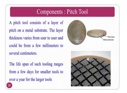
You can see the pitch tool basically pitch tool consist of multiple layers of few millimetres to several centimetres. And normally this pitch is developed on a metal substrate. So, it can be a gas iron substrate it can be a any other stainless steel substrate and many other substrates there will be glues also provided because, this will help the chips that are in micro to nano sizes which are coming out can be accommodated here.
