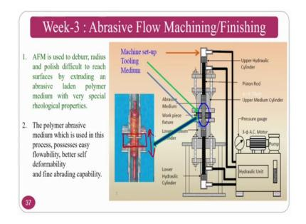
So, abrasive flow finishing process is one of the advanced polymer assisted finishing process where we will use polymer rheological abrasive fluids or polymer rheological abrasive medium. And, you will reciprocate through the workpiece this is the workpiece region and you reciprocate the polymer rheological abrasive medium and you can finish.
