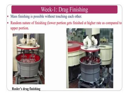
And you can see here how the drag finishing is operating. So, if you can visualise this particular portion that is going to show you how the finishing action takes place in this particular video you can see here the bowl is stationary. But, your component which is fixed to certain entity are rotating about multiple accesses in this way the component can be finished.
