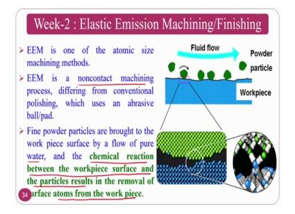
Elastic emission machining is one of the atomic size machining process, but this is the noncontact machining process. So, fine powder particles are brought into the workpiece surface by the flow of pure water and chemical reaction between the workpiece surface and the particles results in the removal of the surface atoms from the workpiece. That means, that the main function of polyurethane ball is to facilitate the particles to come near to the work surface and to pressurise the particles.
