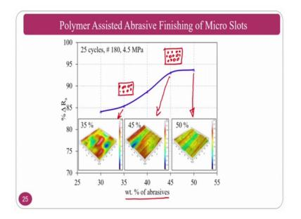
And you can see percentage weight of the abrasive particles. As percentage weight of abrasive particles increases your change in roughness also increasing; that means, that your surface roughness is getting good and good. What is happening here? If your percentage is assume that 35 for a unit area you will have this many number of particles. If you are going to have for 45, what is you are going to have?
