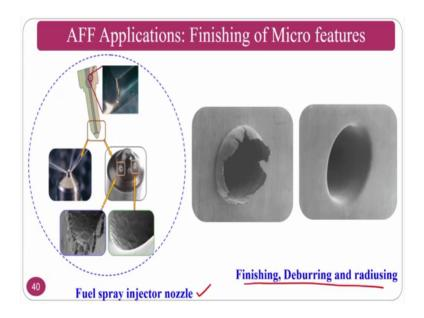
So, the applications, some of the applications not only biomedical applications you can also use for automobile that is fuel injector nozzles, at the same time deburring, radiusing and finishing also we can see. These are all explained in the abrasive flow finishing process itself. Still what I want show here is that you can do the polishing of the micro holes in automobile industry also.
