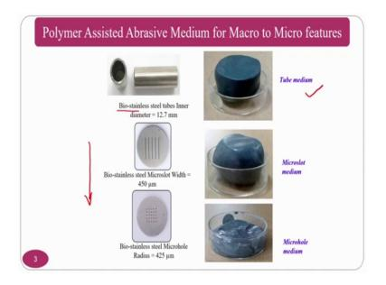
Polymer assisted abrasive medium for macro to micro features; in this what are the few geometries that we are going to do? Practically speaking this is not exactly what we are going to finish the knee implants or hip implants or cardiovascular applications or something, but the preliminary study or preliminary experimentation that we have done at our laboratory is shown here, so that you can understand.
