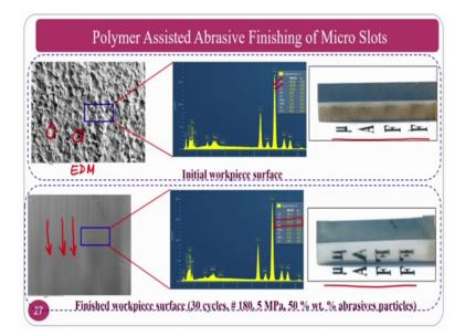
At the same time, you can also confirm this by using elemental analysis that is energy dispersive spectroscopy EDS, can see here the surface EDM surface. It is consist of mostly carbides and iron other things because of which you can see the surface finish
