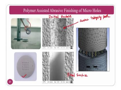
You can see here how the polymer assisted finishing is giving. These are the micro holes a array of micro holes are drilled using EDM process. There is a array tool is there and you are going to generate the array of holes on the surface, that is clearly visible in the bottom picture.
