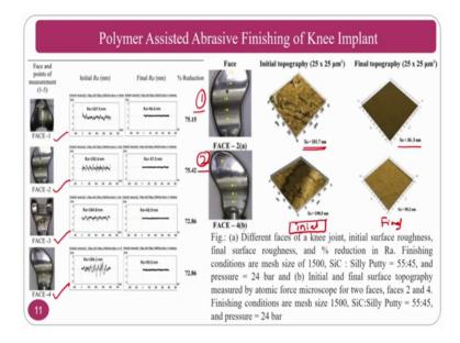
You can see the surface, it is a initial surface roughness which is considered in the normally area surface. It is approximately 182 nanometers, after finishing it is 36.3 nanometers. You can see again at on other side because I said that it has a changing of curvature is there at many many places because of which you have to measure at different locations that is why it is measured two locations here.
