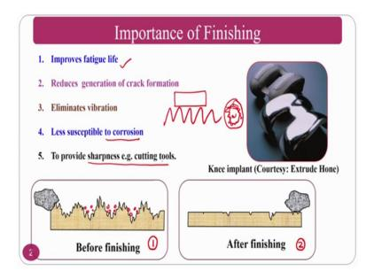
See importance of finishing you should also know what is the importance of machining. It will improve the fatigue life if the surface is roughness is less; that means, that your contact area or bearing area will be high.
