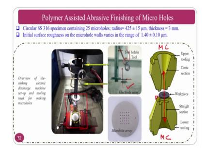
The first thing, how we have generated? The generated using a EDM process that you can see di sinking EDM. A array of micro holes are generated using a array based tool that is clearly visible here. And second thing is you can generate this one, this generated work piece is carried or placed in the fixture and this fixture will be placed in the abrasive flow finishing process.
