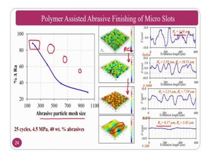
Now, you can see as the abrasive particle mesh size increases; that means, that my particle size is decreasing, this is my particle size, this is my particle size, this is my particle size like that. What is happening here? Your change in surface roughness is decreasing; that means, that you are not going to get much change; that means, that even if for that purpose the research says in this particular graph is if you are going to have a good size of particle.
