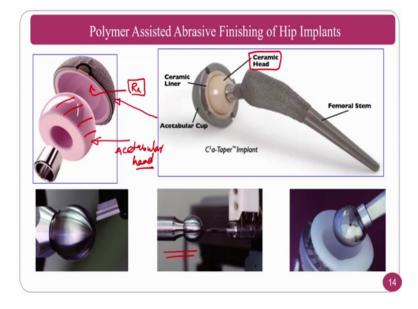
So, in a hip implant acetabular head as well as acetabular socket both are to be properly polished otherwise the relative motion will be not good for the patient. This is acetabular head or normally a it is made up of a ceramic material, at the same time this is as acetabular cup or acetabular socket also we can say. But in acetabular head we mostly bother about the external surface, in acetabular socket we bother about this internal surface, roughness value, so that the contact will be proper.
