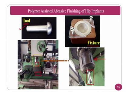
Very simple mechanism is found here and you just have a aluminum tool, and you have a fixture to hold the acetabular socket. Normally, we can design a simple wooden based fixture that can be placed on a milling machine and milling cutter can be replaced by the tool the you can design according to your requirement.
