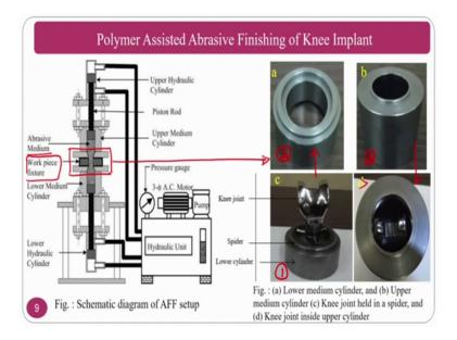
How to polish the knee implant? So, for that purpose we can use abrasive flow finishing process where in you have to play with polymer rheological abrasive medium and you have to design a special type of tooling. This picture is familiar to you because you are going through the abrasive flow finishing process, wherein you have abrasive medium is there workpiece fixture is there. This is the area where you are going to fix your fixture.
