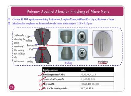
How this is finished? The micro slots are there, this micro slots, the extrusion pressure number of cycles, mesh, weight percentage of abrasives and other things are there, but however, much details are not given here about the medium because medium itself is very complicated as I said. Whenever you are moving towards liquid type of medium what will happen is sedimentation problems will come and this problems has to be overcome by choosing proper rheological additive into the medium, ok.
