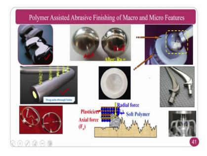
And some of the implants that are finished across the globe you can see here. This is the knee implant which you have seen drug eluting stents. These are the pictures are taken, however, finishing process is under the preliminary conditions; at the same time acetabular socket head, initial surface and final surface.
