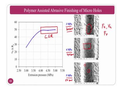
Now, we can see the extrusion pressure effect on the micro hole finishing. If you have the 3 mega Pascal 4 mega Pascal and 5 mega Pascal, the thing is that at low pressures; that means, that your axial force and axial velocity, radial force approximately small compared to your 5 mega pixel. That means, that here 5 mega pixel means 50 bar, 40 bar, 30 bar, in terms of you may see that only it is a difference of 1 mega pixel, but in terms of bar it is slightly higher side.
