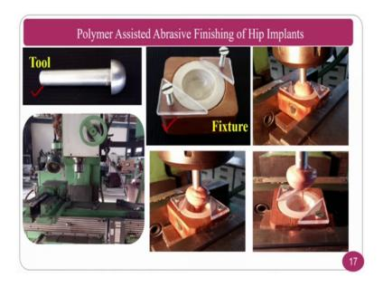
Now, you can see the tool and a workpiece, fixture and other things the tool is here, the workpiece is in the fixture. Now, workpiece is placed beneath the tool and it is filled with optimum amount of the medium that is already optimized its composition, ok. Simple medium is used here however; the people can go for complex mediums and other things.
