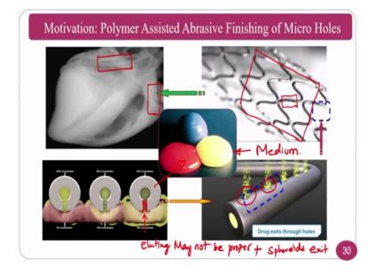
These are all can be done or these are all can be polished using abrasive flow finishing process wherein you have the medium. This particular medium is commercially available by extrude hone company or you can prepare your own medium if you have some polymer technology and other collaborations relevant to this polymer chemistry and other things, ok. This is the polymer medium.
