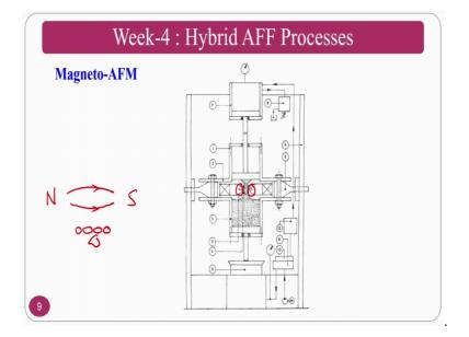
Then hybrid abrasive flow finishing process, this hybrid abrasive flow finishing process also done by Professor H S Shaan and his group out from IIT Roorkee and in this case what they are going to add is they are going to add some of the iron particles such as CIP particles, carbonyl iron particles and they are going to use the North Pole and South Pole.
