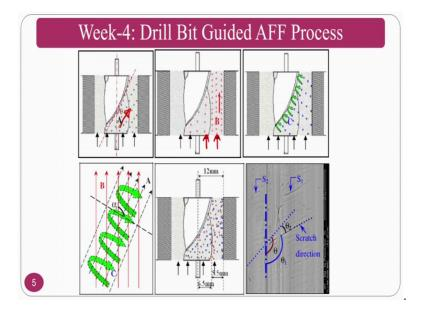
How the various motions can be generated by using this particular process also will be seen in this particular process. So, if you see here what will happen, whenever you are sending the abrasive medium here because of the flute nature this will move along with this direction, at the same time because of the hydrolytic power, it will move axially.
