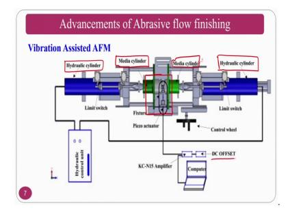
Another advancement is vibration assisted abrasive flow machining process or vibration assisted abrasive flow finishing process, here it is approximately similar to the abrasive flow finishing process only, but the work piece is given vibrations.
