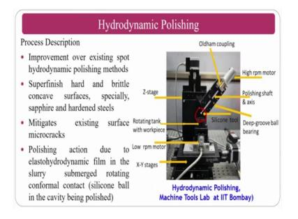
In hydrodynamic polishing; it is similar to the elastic commission machining, but here the contact will be there and you can see here, there will be a ball will be there and you can do the elastic ball. At this elastic ball will have against the work piece surface, there will be a finishing action will takes place.
