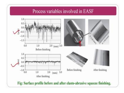
The surface roughness is measured and it is shown that the tubes are better finished and you can see the surface roughness. This is the initial surface roughness and you can see the final surface roughness that at the same time mirror image of the surface is also clearly visible. If at all you want to know about better details about this process, you can go through some of the papers of Professor Suraj.
