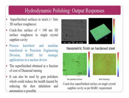
You can see the roughness variations in this one. The superfinished surfaces in steels approximately less than 2 nanometers on the 3D surface and crack free surfaces you can achieve and this is referred and Professor Ramesh Singh as a part of his project has been developed. And you can see the surfaces there is full crack free surfaces after finishing even though crakes are there before finishing process ok.
