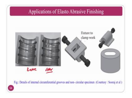
So, some of the applications this is finished using elasto - abrasive finishing process and you can see before and after so much clarity is not there, but if you could have seen the original research paper; then the things may be much clear and fixture for the this type of work pieces are given.
