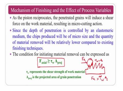
And the mechanism of material removal normally most of the micro cutting in case of any adverse finishing processes will go like this. iIf your axial force is higher than your penetration depth and the cross sectional area of the penetration depth and the shears strength of that work piece material, then what will happen? The micro chip will form if my surface is like this.
