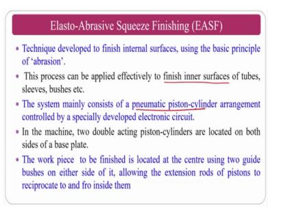
This technique is developed to finish internal and external surfaces and it is effectively for the internal surfaces like tubes and other things. The system mainly consists of pneumatic piston - cylinder arrangement and other things and you have a medium cylinders and you will do the reciprocation with respect to the medium that is there.
