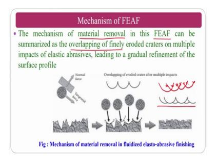
And you can see the mechanism also the elasto - abrasive ball will go and hit the surface and it is like a abrasive water jet machining abrasive jet machining and other things instead of simple abrasive particle here. It is a elastomeric abrasive particle so, that the finishing action will be taken in a nano scale to the micro scale.
