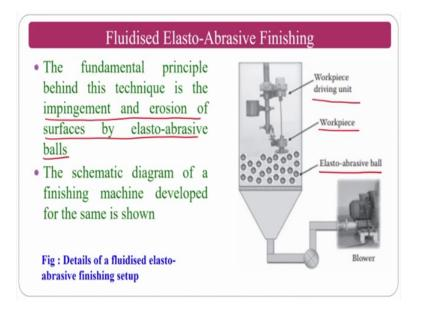
The third variety is Fluidized Elasto - Abrasive Finishing process where in the fundamental principle of this technique is to impingement of erosion of the surfaces by elasto -abrasive balls ok. Schematic diagram is there just, what is elasto - abrasive balls will be there and the work piece is there and work piece driving unit is there so, that the erosion will takes place with respect to the abrasive processes.
