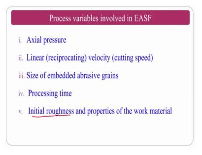
Process variables axial pressure, linear velocity that is nothing, but axial velocity size of the embedded abrasive, processing time, initial surface roughness normally initial surface roughness should be low so, that you will get a better final surface roughness.
