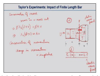
And, if we see in the details in this diagram, so we can see that, first one is the Plastic Wave front, and the second one is Elastic Wave front. Okay. So, this Plastic Wave front, you can see that, this is the plastically deformed area, this area is the plastically deformed area. Plastic Wave front is traveling at a velocity v. And, we know that, this is the area A, the cross sectional area. And, the area is A0, in this portion. This is the area, not the length.
