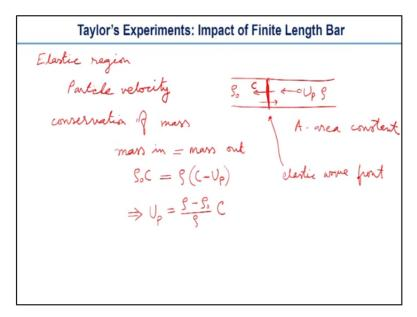
We can draw it here, again. So, the Elastic Wave front, which is moving from right to left, it is C is the Elastic Wave Velocity, and the particle velocity is, we are referring as U p. So now, initially, the mass density is Rho0. But, when the wave travels from right to left, so the right side of this wave front, where the compressed Elastic Wave already passed through, that the density will be little higher. This is the Rho, the other one is Rho0.
