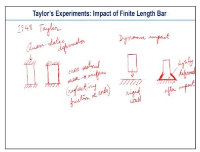
So, Taylor, in 1948, he developed first this experiment, during the World War II. So, Taylor described that, based on a sequence of events, that is, Elastic and Plastic Wave propagation. Before going details about that, we will try to understand, the difference between, Quasi static deformation, and Dynamic impact. So, suppose, we have a Quasi static compression here. This is a cylindrical bar, which is compressed.
