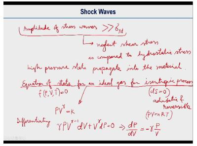
Shock waves are like produced when the amplitude of stress wave greatly exceeds the dynamic yield strength of the materials, so dynamic yield strength of low strength is that yield strength at that strain rate that is which is different than the quasi static or at slow strained, if it is the **if it is** greatly exceeds greater than the dynamic yield stress.
