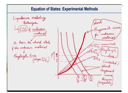
So we will use the impedance matching technique earlier we discuss about that matching technique. So what we will do in this case is, so this is particle velocity Up and this is pressure P, so what we will do is we will draw a curve which is our we call shock Hugonoit curve this is actually shock Hugonoit curve for the projectile that we know that is known material and that is actually the projectile that is known that is for the projectile.
