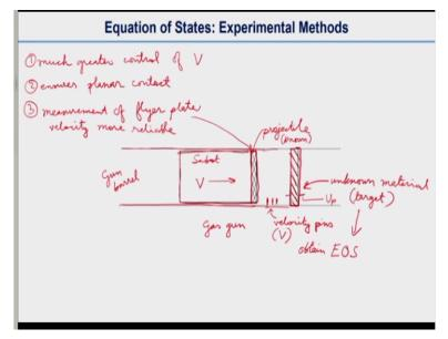
But then we will go and discuss this method because this method is more convenient and then the earlier method, so this is a gas gun system, so this is the gun barrel. So you can see the gun barrel is this is the gun barrel so gun barrel and this is as you know from our earlier classes this we called sabot it is moving at a velocity V and this is the projectile actually this is we can call that projectile or whatever if you have maybe a flyer plate and this.
