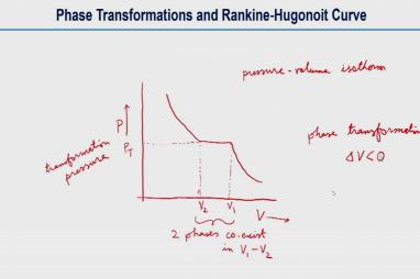
So, we will see first the transformation and with a PV Isotherm is a volume Isotherm that means at constant temperature. So, we have V volume in the x axis and P pressure in the y axis so, for we are drawing a phase transformation that Isotherm on a PV plane. So, the Isotherm we look like something like this. So here, these constant pressures are drawn V 1 V 2. So, these are the volumes had. So, this pressure is corresponding to P T we can write this is transformation pressure.
