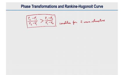
The condition will be P = 2 - P = 1 / V = -V = 1 - P = 1 - P = 0 / V = 1 - V = 0. So, that is the condition that is the condition for 2 waves 2 Shock Wave structure. If that does not satisfy that means the second shock wave will overtake the first or that means, now, it will be only 1 Shock Wave instead of 2. So, with that, so, we are closing for today. So, we have discussed about pressure volume, Isotherm and Rankine-Hugonoit Curve.
