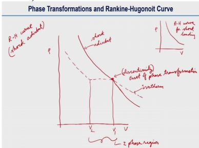
So, we will see it in 2D plot which will be easier for us to visualize. So, the early plot was complicated because we have even temperature axes. And so, now here we have in a simple PV plot, the same case, same idea bit here. We can call Rankine-Hugonoit Curve or even it is known as shock adiabat because it is adiabat process shock adiabat on a PV plane, so, first we will draw this on the Isotherm what we got in the earlier curve.
