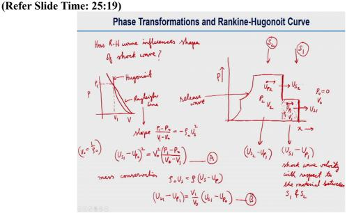
So, now you will check how this Rankine-Hugonoit Curve influences the shape of this Shock Wave how R-H curve influences shape of Shock Wave so, for that we need to draw a draw shock front shock front of 2 waves. So, what we will do is will draw a shock front of 2 waves the wave one we will write this wave as S 1 or you can just say this wave is S 1, Shock Wave 1 and this wave as S 2 the Shock Wave 2.
