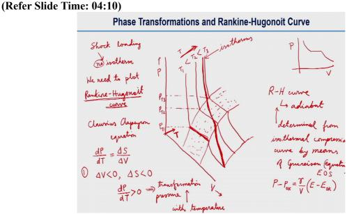
So, now in case of shock loading, so, we do not have the Isotherm. Isotherm shock loading we do not have the Isotherm. So, I will write no Isotherm because the temperature will change and so, we need to develop we need to plot the Rankine-Hugonoit Curve for this shock loading Rankine-Hugonoit Curve. So, we will see how to draw that. So, what we will do is we will try with the earlier whatever the previous slide.
