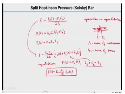
So now we will try to get the stress out, so what will be the stress as we know the specimen is in equilibrium. That means you have a specimen and these are the bars and this is the specimen. If you take any section in the specimen that you will get the same stress and that will lead you to the average force divided by area will be equal to stress.
