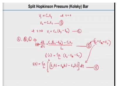
V1 will be equal to C0 epsilon I, related to incident wave that is that time T = 0, so we will get to know what will have happen after time t = 0. And then V2 will be equal to C0 epsilon related to the transmitted wave. So from here we will try to find out these stress and strain. So as I told so at time t equal to greater than 0, the V1 will be changed because a reflected wave will also contribute to it, that will give like epsilon I - epsilon R.
