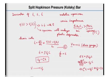
So we can get the stress strain relation here the derivation of sigma stress epsilon strain and epsilon dot the strain rate. Let us assume that we have a metallic specimen and we will assume that the sonic impedance of the bar that will be rho0, A0, C0 will be greater than the sonic impedance of the specimen. As you know the sonic impedance has also the area term sometimes we discussed earlier that only rho and C0 we earlier discussed as rho  $\mathbb{C}$  C.
