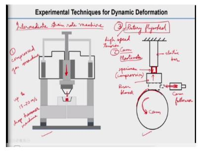
So we will now talk about the intermediate strain rate machines intermediate anyways these terms are very relative. So intermediate strain rates probably you can define as like which are not like in the very slow strain rate like quasi static rates. And which is also not very high strain rate like you know an explosive test was similar high strain rate experiments.
