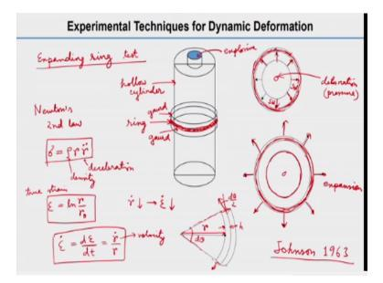
Another important test is expanding ring test or technique it is, so the ring is somewhere here 13 ring, this is the ring. And we have a hollow cylinder let us say it is a it is made up of steel and then we have explosive which you want to detonate to produce the deformation in ring. So there are 2 another rings up and down these are guard, so what will happen is these if you see the top view of this.
