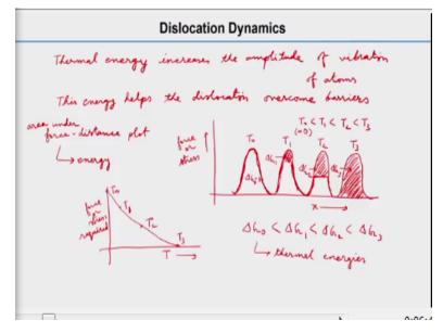
So the thermal energy increases the amplitude of vibration of atoms as we have discussed even earlier the atoms are vibrates continuously. So this thermal energy can increase that amplitude of vibration. So this energy can help the dislocation to overcome the obstacles or the barriers. So we will see just by plotting this, so in this in the x axis we have X that is distance and then in the y axis we have force or stress.
