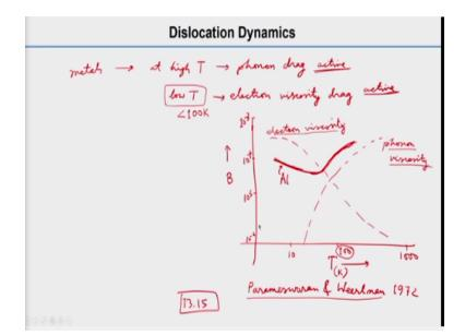
And that you know for metals we should understand that for metals at high temperatures at high T. So phonon drag mechanism will be active and at low temperatures that electron viscosity **be** drag will be active viscosity drag, so I would write active ok, so active. So we can see with the help of a plot that is mostly from 1972 publication by Parameswaran and Weertman 1972.
