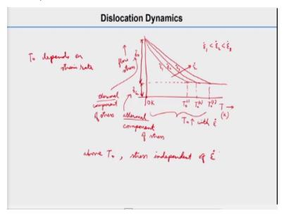
So this earlier relation we can have a plot related to that, so this plot is temperature in the x axis let us say temperature in Kelvin and then we can have flow stress on the y axis flow stress. So we will see this at different strain rate, so what will happen is this is one strain rate, this is another strain rate and this is another strain rate. So let us say first one is epsilon dot 1, epsilon dot 2 and epsilon dot 3.
