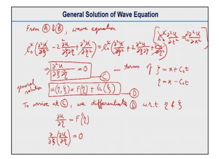
So, from A and B, if we substitute in the Wave Equation, and the Wave Equation will be, C0 square. So, the Wave Equation, we have is, C0 square. This, is equal to, second partial of U, with respect to X. So now, we will write the Wave Equation, from A and B, using the relation, we got an A and B. So, that will be, something like this, twice, plus, this is second partial, is equal to C0 square, plus second partial of U, we just picked the second variable.
