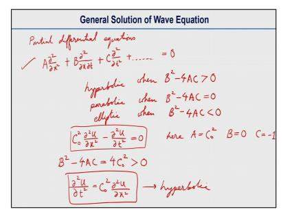
So, we know, that the partial differential equation equations of the form, A double-partial, with respect to X, B double-partial, with respect to X and T, plus C double-partial, with respect to T, plus ..., equal to 0, are classified into Hyperbolic, when B square minus 4AC, is greater than 0. And, Parabolic, when B square minus 4AC, is equal to 0, and elliptic, when B square minus 4AC, is smaller than 0.
