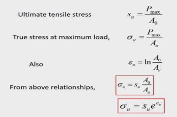
But in this we found that ultimate tensile strength where the maximum load is there you have calculate, you wanted to find out the relationship between this true stress at maximum load. So ultimate tensile stress is given by say Su given by P max what is the maximum load by  $A_0$  when the true stress at maximum load sigma u is the P max by Au where you should know what is the initial cross sectional area.
