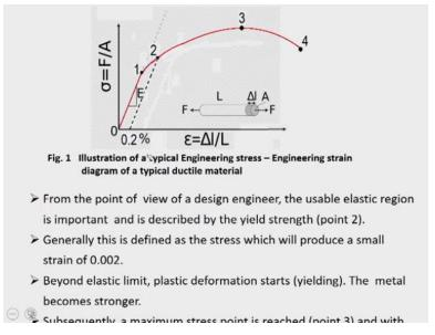
So from point 2 the yield strength keeps on increasing. So when you unlock the specimen at any point beyond 2 you will find that there is a permanent deformation takes place and with the more and more straining this permanent deformation keeps on increasing. Because initially you know whatever was the elastic energy absorbed that will always determine constant but you will find that the stress necessary for plastic deformation that keeps on increasing with the increase in strength.
