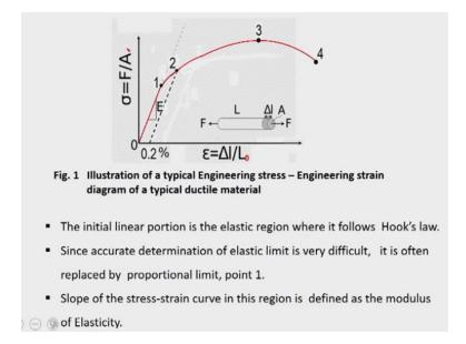
So that is the e value you can calculate by L / L naught – 1. So this is how you get a typical stress strain curve. So in this when you look at it, what we can see is that the initially there is linear path so this load versus elongation plotting it you will get the same type. Only thing is that here the stress divided by area and the strain by delta L / L when you are doing it you will get this type of a plot.
