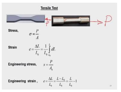
So this is the round bar say a uniform round section is the cylindrical piece is there at the center portion you have a reduced cross section with a some radiuses are given, as per the ASTM standards you get the standard dimensions for this if you are conduction a test you follow some standards, generally, throughout the people follow this ASTM standard though in a European countries you know they also have different standards and other thing.
