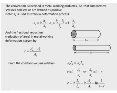
So convention is reversal metal working problem, so that the compressive stresses and strains are defined as positive okay. So you define it as positive and then you do the analysis, only thing is that it does not matter whether it is compressive or tensile what matters is what is the amount of strain you have given in plastic working of metal that is why so there is not going to be much only thing when you do the calculation you have to be very careful what you are taking it.
