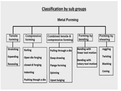
Now you have classification by subgroup the metal forming process. So, one is tensile formation where you are have stretching expanding and recessing you have compressive forming examples are rolling, open-die forging, cross die-forging indenting, indentation is another process of compressive process pushing through a die. So that is the extrusion combined tensile and compressive forming is there pulling through a die, deep drawing, flange forming.
