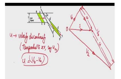
Now for this particular case, let us draw the velocity diagram. So because for this to be kinematically satisfied admissible, then we have to draw the velocity diagram which is called as holograph, so let us see that. The absolute velocity, the initial velocity it is moving with a unit velocity, so you can just star with origin O and then let us give to some scale of the velocity you draw a unit velocity with 1 okay. So, this is that value.
