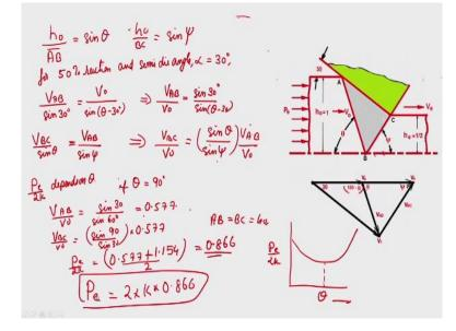
Now this you can calculate either by measuring from this velocity diagram, from the hodograph, or you can do it by analytical method also or from physical method also. However, it is easier to evaluate it by analytical method because you can just take h0 by AB = sin theta and then h0 by BC = your sin psi okay. So from that if you do it for a 50% reduction and semi die angle alpha = 30 degree. Applying law of sin you can say V Star AB or VAB by sin 30 degree = V0 by sin
