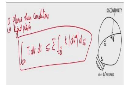
Now in the same thing assuming that plane strain condition, so I am not going to too much depth in that planes because we will with the practical situation, we will just discuss with that case following this, so that is why. Assuming the plane strain conditions and material is rigid plastic, that is where the material consists of rigid blocks of material separated by lines of tangential displacement discontinuity.
