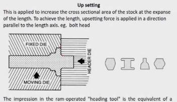
The impression in the ram-operated "heading tool" is the equivalent of a hammer or press top die. The "grip dies" contain the impressions corresponding to the hammer or press bottom die. Grip dies consist of a stationary die and a moving die which, when closed, act to grip the stock and hold it in position for forging. After each workstroke of the machine, these dies permit the transfer of stock from one cavity to another in the multiple-impression
