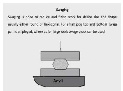
Then is the swaging. Swaging is done to reduce the finish work for desired size and shape, usually either round or hexagonal shape they obtain for that the swaging, may be to some extent there is the die cavity is there, so you get the very good shape for that. For small jobs, top and bottom swage pair is employed, whereas for large works swage block can be used. (**Refer Slide Time: 45:02**)
