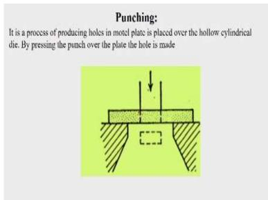
Then there are punching operation. The metal is kept on a die and this is the work piece material, it is kept on a die and punching tool no it moves downward and then causes shearing of the material resulting in a small die. Depending upon the shape of the punch, you will get a hole which is made there, so that is the punching operation which is done.
