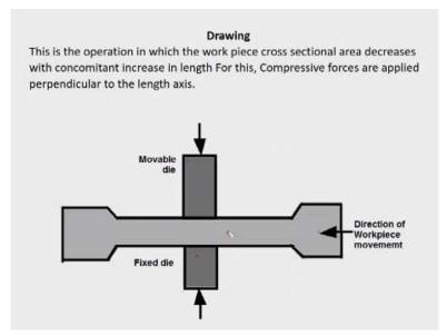
Say first is drawing operation. So this is your work piece material and then it is kept between on the top of a fixer die and then a mobile die is there which will be pressing. Now depending upon the shape of this, if the shape is concave like this what happens is that the material will flow perpendicular to the direction of the mobile die, movement of the die okay, so it move laterally and then it gets elongated.
