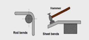
Then there are bending operation, normally which is done with the help of a hammer. If it is sheet bending, you bend it, or if it is a rod you can bend it on a roller and get the shape.
