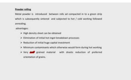
There is another when you called about rolling, there is also something called as powder rolling. In this the metal powder maybe metal means even it can be pure metal or it can be alloy powder. They are introduced between the roll and then, okay, it is compact and when it passes through between the roll and gets compressed. So, here it gets compacted into strips you will get green compact or green strips.
