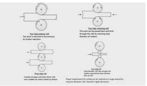
So, let us come to the type of rolling mills, when you say the most simplest material is the twohigh pullover mill, rolling mill, two-high pullover mill is what you are getting here. Okay. So, in this two counter rotating rolls are there with a proper roll gap between them. Okay, and then what happened to them the strip enters from one end and then, Okay, you will find that with the initial thickness the initial thickness is here the final thickness is something something around here.
