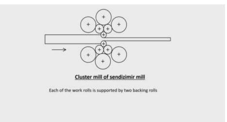
So, in that case, so you have a large number of rolls. So, each roll is supported by two back end rolls. So, when you look at this working roll is supported by two back end roll here, whose diameter is larger. Because if it is, in the previous case know, only one support roll is there. So it may shift this side, the other way. So whereas in this particular case between these two backing rolls you know, that gap is there.
