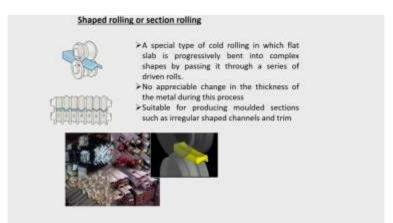
And you can get a special type of cold rolling in which flat slab progressively bent into complex shapes by passing it through a series of driven rolls are also you can get different shapes also see like this step shapes. Now you will find that the roof tops thin sheets roofs are also there. Corrugated shape these are all obtained by this section rolling strands. So you can get different shapes.
