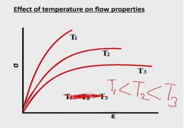
Figure showing the effect of temperature on flow curve
