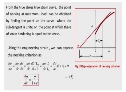
Now, let us look at how to determine this value from a stress strain curve so the true stress true strain curve the point of necking at maximum load can be obtained by finding where the sub
