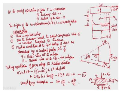
Say for example, if I just take that, this is a platen and this is a platen and in-between know you have your work piece material. When it is deforming you know there will be a barreling. So, the shape of a barrel is coming and you are having applying the force here and in the maybe in normal cases the bottom platen will be a fixed plate ok.
