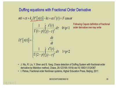
In addition to duffing equation what you have seen before. So, we can have different other type of duffing equation. So, here is one duffing equation duffing equation with the fractional order derivative. So, here these additional term you can see. So, that is known as the fractional order. So, you can study many different type of duffing equations and their response and which will lead to many different type of bifurcation points also.
