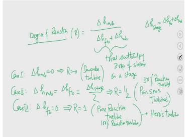
So, you can understand that not only in the nozzle, but pressure also drops in the moving blades. So, when pressure drop takes place both in the moving blade as well as in the fixed blades that is fine because this is nozzle shape.
