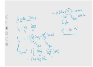
So, you know that for the impulse turbine, this velocity ratio  $v_r = \frac{v_b}{C_1} = \frac{\cos \alpha_1}{2}$ . Now for this particular velocity ratio; diagram efficiency maximum is nothing but  $\eta_D = 2(v_r \cos \alpha_1 - v_r)(1 + K_b)$
