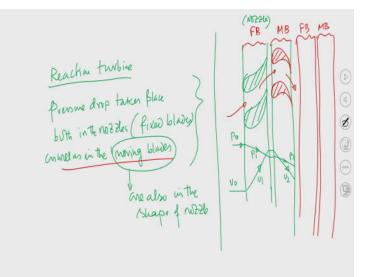
So, we have seen in impulse turbine, entire pressure drop takes place in the first row of nozzle. There is no pressure drop of steam when it is passing through the passage between two blades, but in case of a reaction turbine pressure drop takes place both in nozzles and sometimes known as fixed blades and as well as in the moving row of blades.
