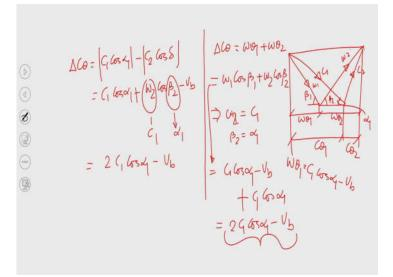
So,  $\Delta C_{\theta} = C_1 \cos \alpha_1 - C_2 \cos \delta$ . So,  $C_2 \cos \delta = w_2 \cos \beta_2 - v_b$ . This is from  $w_{\theta_2} - v_b = C_{\theta_2}$ . So, this is  $w_2 \cos \beta_2 - v_b = C_{\theta_2}$ .
