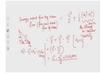
So, energy input per unit mass flow of steam is nothing but  $\frac{C_1^2}{2}$  + for the impulse turbine, we have seen this is only the energy input; but in case of a reaction turbine, on the top of that we are also having the reaction force and that reaction force is developed only because of the reduction in relative velocity.
