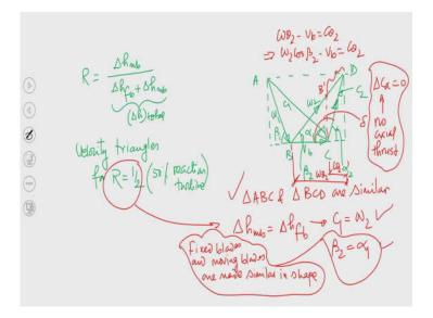
So,  $R = \frac{\Delta h_{mb}}{\Delta h_{total}}$ . Now, we are trying to draw velocity triangles for R = 0.5. So, this is  $v_b$  that is blade velocity and this is the inlet velocity diagram. Now, this angle is  $\alpha_1$  and this angle is  $\beta_1$  that is what we have seen in the last class. Now, this is inlet triangle. What about the outlet velocity triangles? This angle is  $\alpha_2$  and this angle is  $\beta_2$  and say this is D. So, this angle is  $\delta$ .
