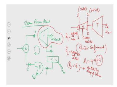
So, if we try to draw the schematic diagram of the steam power plant; there is a boiler and this is turbine, and after doing work steam leaves from the turbine, it is taken to this heat sink wherein upon rejecting heat, the working fluid is again taken for the next cycle.
