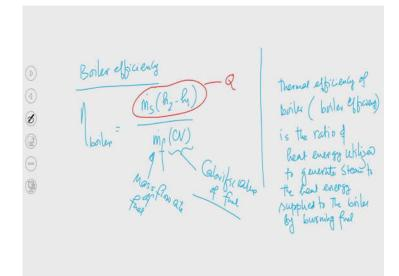
Now, having established this, we can understand what boiler efficiency is. For the conversion of water into steam; for this phase change, amount of energy required is  $h_2 - h_1$ . If we try to write total heat, it will be  $\dot{m}_s (h_2 - h_1)$ .
