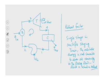
So, we have this is boiler where heat is added and finally, heat is getting rejected from the condenser. To have the cyclic process from this plant, we must have a heat source and one heat sink and that is to satisfy the second law of thermodynamics.
