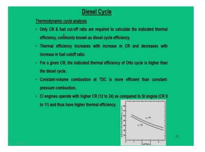
So, this is the some summary is that when you do this diesel cycle analysis, we require the compression ratio and fuel cut off ratio to calculate the diesel cycle efficiency. Thermal efficiency increases with compression ratio and decreases with increase in the fuel cut off ratio.
