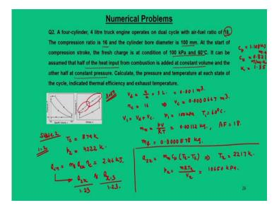
And, in the similar logic we have another problem that is four-cylinder, 4 L truck engine that operates in a dual cycle here the air fuel ratio is 18, compression ratio is 16, and bore diameter is 100 mm, in intake condition is 100 kPa and 60 °C, but the entire idea is that heat addition process. So, total heat addition process is divided into two halves. So, the first half is at constant volume and second half is at constant pressure and both amount is equal.
