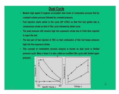
Then, we will move onto another cycle which is dual cycles. So, people think of that how we can improve the efficiency of Otto cycle at the same time; we can approach the efficiency of diesel cycle, just by doing some alteration in the heat addition process.
