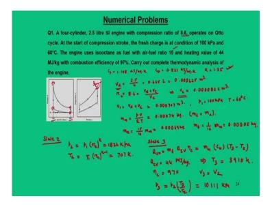
So, with this we conclude the end of the lecture. Now, let us solve some numerical problems based on these study what we have done so far. So, the first problem which I am going to discuss is consider a four-cylinder 2.5L SI engines with compression ratio 8.6 and it operates on Otto cycle. So, basically this is an Otto cycle analysis. So, you we have to use all thermodynamic equations of Otto cycles.
