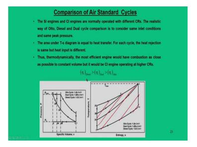
The another way of comparison is that is that based on the same inlet condition and same peak pressure and temperature, what does this mean is that normally the engines are operated in different compression ratio. So, the realistic approach for them is to consider the Otto, diesels and dual cycles for same inlet conditions and same peak pressure and temperature.
