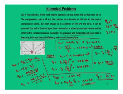
So, this is all about the thermodynamic state pressure and temperature of the cycle.
