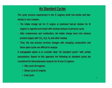
So, let me give you some brief introduction about what the air standard cycle means. Ideally, when you look at Carnot cycle, we need a working fluid to run the engines. In a similar sense, when you discuss about SI engine or CI engines, there are working fluids which are very specific to those engines. For example, in SI engines petrol is the base working fluid, for CI engines diesel is the base working fluids.
