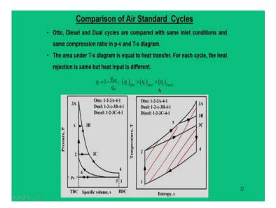
Now, next approach is to compare the air standard cycles. One way of comparing them is that for same inlet conditions and same compression ratio. So, we have pressure volume diagrams and temperature entropy diagrams. So, what we are making constant is for same inlet conditions.
