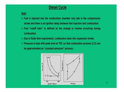
But, some important analysis here we are going to make here, that the assumption of constant pressure process, because fuel is added into the air. So, that it is not possible to maintain the constant volume process when fuel is added.
