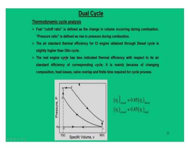
So, whatever I have explained this is shown here, one is the fuel "cutoff ratio", other is the "pressure ratio", that takes part into the calculation of thermodynamic cycle efficiency. The air standard cycle of CI engines is obtained through diesel cycle is higher than that of Otto cycle, but here we must remember the diesel cycle operate at higher compression ratio. Whereas, Otto cycles operate at, lower compression ratio; so, this is the reality.
