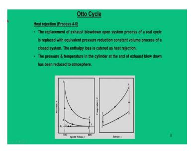
Then, we have heat rejection process. So, that is regarded as a constant volume processes from 4 to 1, and this happens close to BDC or mostly at BDC. And, this 4 to 1 is represented in the temperature entropy diagram like this. So, it is a constant volume process.
