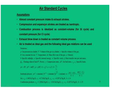
Now, we will consider about the assumptions that are involved in our calculations. We also have to give a thermodynamic meaning about the processes that are encountered in the IC engine. So, first assumption in that line is that, the intake and exhaust strokes are constant pressure processes.
