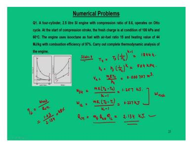
For state 4  $T_4 = T_3 \left(\frac{1}{r_c}\right)^{k-1} = 1844K; p_4 = p_3 \left(\frac{1}{r_c}\right)^k = 554$ kPa; $V_4 = \frac{m_m R T_4}{p_4} = 0.000707$ m<sup>3</sup>
