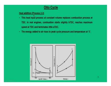
Next is the heat addition process. So, we have already explained that heat addition in a SI engine process can be best approximated, when it is considered as a constant volume processes. So, that means, point 2 to 3, we can regard it as a constant volume processes, when the piston is exactly at TDC, but in reality you will find that the combustion starts slightly before TDC and it reaches maximum speed at TDC and then terminates little after TDC.
