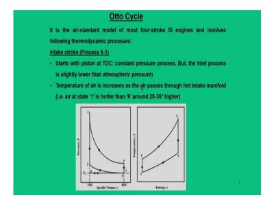
So, let us start with the first cycle that is Otto cycle. The air standard model for a fourstroke SI engines is considered for Otto cycle. So, it starts with an intake stroke as you see in this figure there are two types of diagram, which is represented; one is pressure volume diagram, other is temperature entropy diagram.
