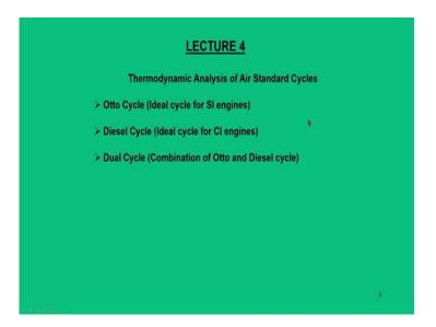
So, in this lecture we are going to discuss about three important cycles; one is Otto cycle, which is an ideal cycle for SI engines, diesel cycle which is an ideal cycle for CI engines, dual cycle which is a combination of both Otto and diesel cycle as far as the combustion mechanism is concerned.
