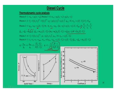
So, here we can see that all equations follow the similar one as we do in the Otto cycle, but only difference that we can see is the heat addition process. That is while calculating  $q_{2-3}$  the heat input we are using  $c_p$  here instead of  $c_v$ . And, since it is a constant pressure process, it also incurs the work transfer  $w_{2-3}$  and also we define a parameter fuel cut off ratio that is  $\beta = \frac{V_3}{V_2}$ .
