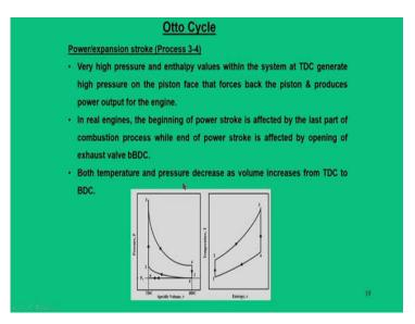
Then, we have power strokes. So, after the combustion process is over. So, pressure and temperature gets increased. So, the piston phase sees a force acting on it. So, in this process the piston starts moving again from TDC to BDC. So, we call it as a power strokes.
