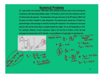
$$\eta_t = \frac{T_8 - T_9}{T_8 - T_{9s}} = 0.85 \Longrightarrow T_9 = 786.8 \text{K}$$
