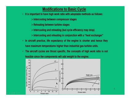
So, for that reasons, there are some adoptable or possible methods that are introduced, first thing is a intercooling between compressor stages, and reheating between turbine stages. So, these two are things that basically to increase the work ratio that is we need to either increase the work output from the turbine side. So, that can be done by through reheating, other way is that you can reduce the compressor work. So, that can be done through intercooling.
