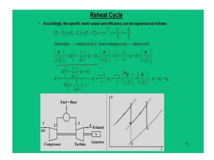
And, work transfers for HP and LP turbines are equal. And, the another way of representing the cycle efficiency the way we represented for basic cycle and heat exchange cycle, we can also calculate for a reheat cycle. What can be the expression for non dimensional work in terms of pressure and temperature ratio?
