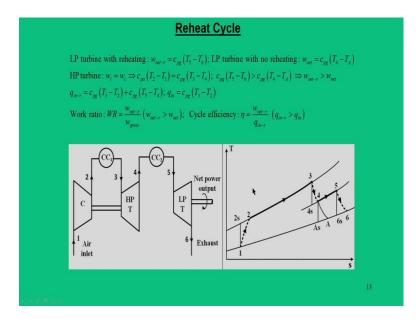
Now, let us see that how reheat improves the work ratio and what happens to cycle efficiency? So, this phenomena is something a reverse phenomena. So, let us think about low pressure turbine with reheating. So, here the power output has two parts; one is the actual power that we get from low pressure turbine and the high pressure turbine normally drives the compressor.
