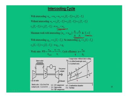
Now, let us see that how an intercooling cycle mathematically proves that work ratio is increased and cycle efficiency drops. So, we can see the circuit with an intercooling circuit, the work input would be  $w_{in-i} = w_{12} + w_{34}$ ; that means, these are the two circuits that consumes work.
