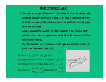
And, to get some mathematical assessment, we define a parameter called as a heat exchanger "effectiveness". And, it is defined to allow the temperature difference necessary for heat transfer or transfer of heat that is ratio of heat received by the air to the maximum possible heat which could be transferred from the gases in the heat exchanger.
