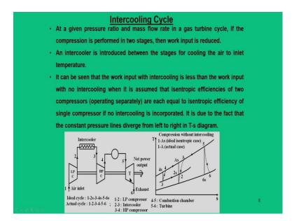
Now, let us start with the first modification that is what we call as a intercooling cycle. So, it has been shown in thermodynamics, that when you make this compression process in a quasi static manner we will consume less work. So, in that sense instead of going for a single stage compression. a intercooling method is adopted.
