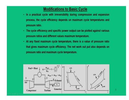
But, that has also limitations because the practical cycles are associated with irreversibility and second issue is that the upper limit of the cycle temperature is fixed based on the materials used in the turbine blades.
