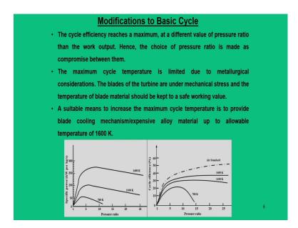
And, then another topic of interest which we discussed in the last class is that the specific power or power output and cycle efficiency, they are functions of pressure ratio as well as the temperature ratio.
