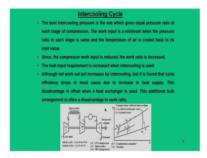
Now, there are some other factors that plays when we will deal with the compressor; in the last module, we will find out that the best intercooling pressure is the one which gives the equal pressure ratio at each stage of the compression.
