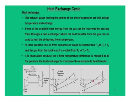
Now, we have already discussed some details about heat exchange cycle, but here the heat exchange cycle is analyzed with a context that, the heat exchanger has to be a integral part when you are talking about reheat or intercooling.
