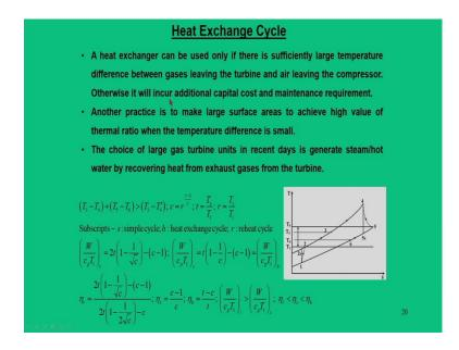
So, it is also possible to say that how heat exchanger cycle improve the cycle efficiency. So, a typical T-s diagram is drawn here. So, from this we can say that for a heat exchange cycle that is efficiency is defined by  $\eta_h = \frac{t-c}{t}$  and by putting this we can say, this particular relations holds good  $\eta_r < \eta_s < \eta_h$ , that is for a heat exchange cycle the efficiency is always higher. Of course, we are not touching the work output.
