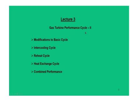
So, under this lecture following topics will be discussed that is modifications to basic cycles. First we will discuss about intercooling cycle, we will discuss about a reheat cycle. And, these two cycles are introduced in the basic cycles with a main intention to increase the work ratio or work output.
