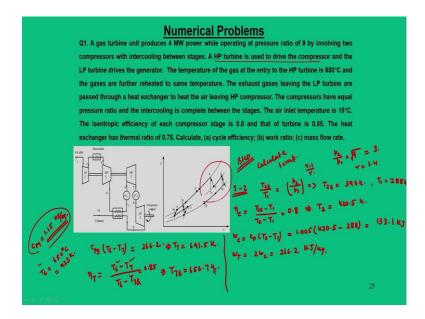
So, the problem goes like this that a gas turbine unit produces 4 MW power, while operating at pressure ratio of 9 and it involves two compressors with intercooling in between stage.
