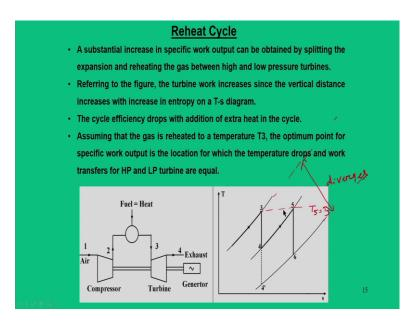
So, this is again another way of representing the things and some better inferences that we can draw that substantial increase in this specific workout can be obtained by splitting the expansion and reheating of the gas between high and low pressure turbines. So, because of this turbine work increases since the vertical distance increases, with increase in the entropy in a T-s diagram. Because this particular gap, as you go further in the T-s diagram, this part diverges.
