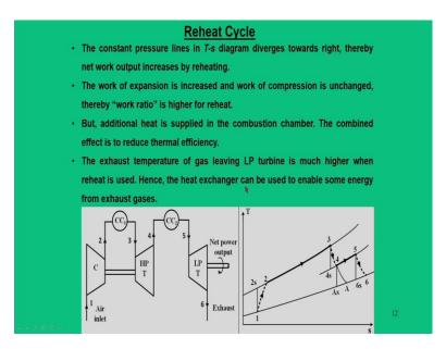
And, in the process of this reheating what we get the expansion work is increased, but since the compression work remains unchanged. So, the work ratio is always higher, but the additional heat is supplied in the combustion chamber. So, the combined effect is to reduce the thermal efficiency.
