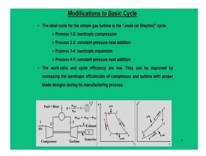
Just to give you brief introduction about the basic cycles with what we discussed. The simple gas turbine or Brayton cycle has 1-2 isentropic process, 2-3 constant pressure process where heat is added, 3-4 isentropic expansion process in the turbine and 4-1 constant pressure heat rejection process.
