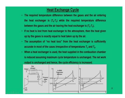
Some of the other inferences that can be drawn here, that required temperature difference between the gases and air entering the heat exchanger is T6 minus T2, while the required temperature difference of the gases and the air leaving the heat exchanger is T5 minus T3. So, the heat is lost from the heat exchanger to the atmosphere, then the heat given by the gas is exactly equal to the heat taken up by the air.
