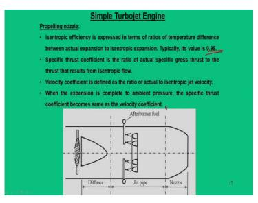
Let us see how you are going to get. This first the isentropic efficiency is expressed as the ratio of temperature difference between actual expansion to isentropic expansion and its value is typically 0.95. Whereas, specific thrust coefficient is nothing but the ratio of actual gross thrust to the thrust that is resultant from isentropic flow. Had the flow have been isentropic what would have been the thrust.
