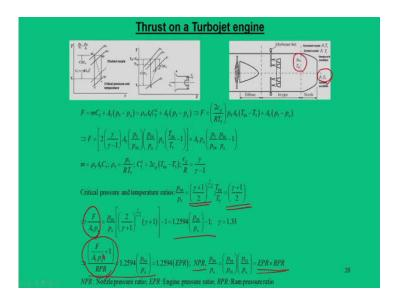
So, how it is calculated. So, thrust is basically two parts: jet velocity plus the pressure drag that is  $F = mC_5 + A_5(p_5 - p_a)$ . Now, putting this value mass flow rate as  $\rho AC$ , we can get this particular expressions  $\rho_5 A_5 C_5^2 + A_5(p_5 - p_a)$ .
