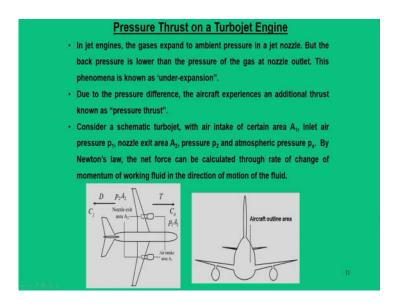
Now, moving further, we are going to discuss on the pressure thrust on a turbojet engines. In fact, in previous lecture, we discussed this pressure thrust and that concept was typically different in a sense that there we defined 3 pressure ratios, one is nozzle pressure ratio, one is ram pressure ratio, and we found out a non-dimensional thrust coefficients as a function of nozzle pressure ratio.
