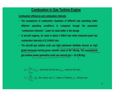
The other term that is also important is nothing but the combustion intensity. Now, if you want to compare two combustion chambers, another way of quantification is that combustion intensity that is  $C_I = \frac{Q_R}{V_c p_{in}}$ ; where,
