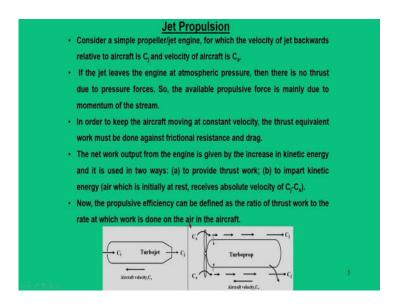
Now, let us do a very simple analysis whether it is a propeller or jet engine for which there is a velocity of the jet which is defined as  $C_j$  and the velocity of the aircraft which is  $C_a$ . So, you can see here, the  $C_j$  is your jet velocity whereas, aircraft velocity is  $C_a$ . And similarly, same thing happens here also for turboprop engines.
