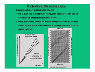
And if you give some typical numbers for this, the air fuel ratio in a gas turbine engines is 60 to 120 whereas, in our IC engines it is 14.5 that is stoichiometric air fuel ratio. Air velocity at the entry of the combustion chamber is limited with 75 m/s because if you keep on increasing the airspeed, we do not have sufficient mixing time. So, to the best available technology till today we say that the air velocity at the entry to the combustion chamber is limited by 75 m/s.
