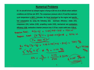
And last segment that we are going to calculate is about specific thrust. So, here there are two parts, one is momentum thrust and pressure thrust.
