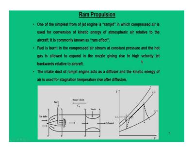
Another concept that drops in from this jet is what we call as a ramjet engine. So, it is simply a ramjet engine, in which the compressed air is used for conversion of kinetic energy of atmospheric air relative to the aircraft. And we call this as a ram effect.
