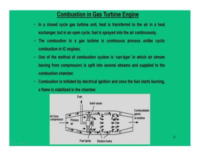
And the last segment of this aircraft propulsion or in fact, in gas turbine engines is combustions. And we have covered all the components, turbine, compressor, intake, nozzle, all these components are covered, but we have not discussed anything on how the combustion process happens in the gas turbine engines.
