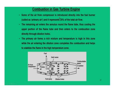
And some of the air from the compressor is introduced directly. So, we call this as a primary air. And it is only about 25 percent of the total air. The remaining air enters to the annulus or through these dilution holes, and in the flame tube. The primary air forms the rich mixtures and temperature is high in this zone. So, while air entering the dilution zone completes the combustion and it helps to stabilize the flame in the high temperature zone.
