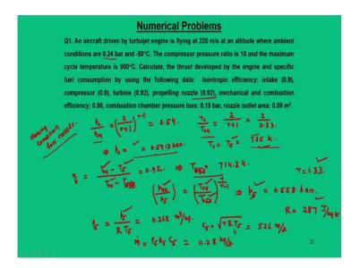
And for this reason again, we have to calculate choking condition for nozzle.
