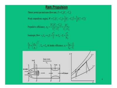
So, a brief calculations in this aspect we can have here is that the thrust power per unit mass flow rate which you can calculate  $F = C_a \left( C_j - C_a \right)$ . So, from this, we can get also work output from the engine that is  $\frac{1}{2} \left( C_j^2 - C_a^2 \right)$ . So, based on this, we define this propulsive efficiency.
