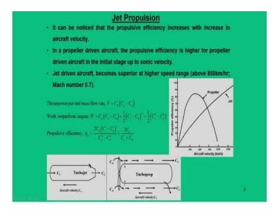
From this, a simple relations can be made that thrust power per unit mass flow rate that is  $F = C_a \left( C_j - C_a \right)$ . So, that work output from the engine becomes W that is nothing but  $\frac{1}{2} \left( C_j^2 - C_a^2 \right)$ . So, you can say propulsive efficiency this can be defined by  $\frac{2C_a}{C_j + C_a}$ .
