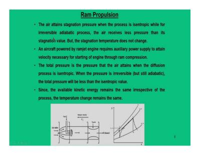
Other concept that are used here that air attains the stagnation pressure when the process is isentropic and in fact, this duct is typically an adiabatic duct, where the air receives less pressure than the stagnation value. But whatever the case may be, the stagnation temperature does not change, that is 1 and 2, the stagnation temperature does not change.
