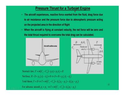
So, let us do this calculations that from the Newton's law, we can say how much force that acts on the aircraft that is through the jet and from the pressure force. And that is nothing but your reaction force. So, the net force becomes reaction force minus drag and plus this pressure with respect to this aircraft outline area;  $R - D + p_a (A_1 - A_2)$ . So, from this we get an expression for drag which is which is nothing but  $D = R + p_a (A_1 - A_2)$ .
