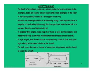
So, previously in the our last lecture, we discussed about the a jet engine and it is divided into two broad categories, one is turbojet engine, other is turboprop engines. So, in a turbojet engine the thrust is developed through a propelling nozzle, we call this as a jet.
