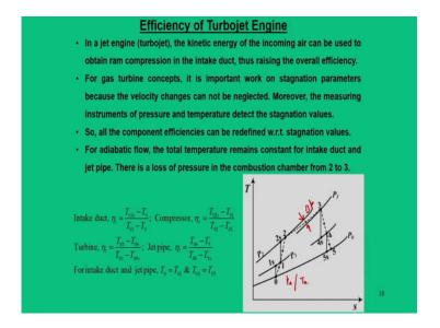
Apart from this, let me discuss some other thermodynamic aspects that we typically define for isentropic efficiency and with respect to a turbojet engine. So, in earlier situations, when we define this as efficiency, we normally do not encounter or do not take into account about the kinetic energy or potential energy change in our temperature or pressure calculations.
