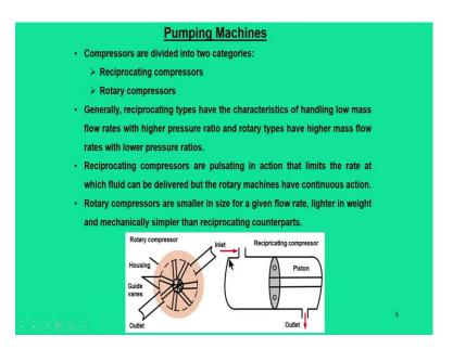
There are two broad categories of pumping machine, one is reciprocating type, other is rotary type. So, if you can broadly see this figure that there is an inlet, there is an outlet. So, what we can see is that during the suction stroke in a reciprocating compressors, the air gets into the cylinder, and it gets compressed and finally, there is a outlet in which gas is discharged.
