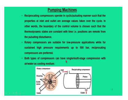
The reciprocating compressors operate cyclic or pulsating manner such that properties at the inlet and outlet at the average values taken over the cycle. And the boundary of the control volume is chosen such that the thermodynamic states are constant; that means, positions are remote from the pulsating disturbance.
