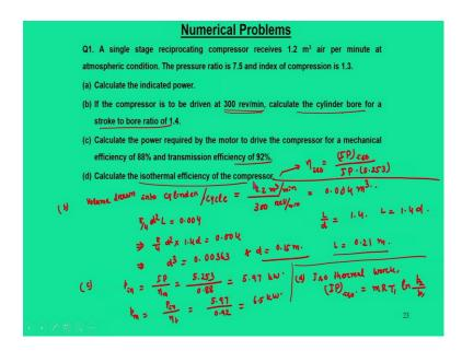
If the compressor is driven at 300 revolution per minute, we have to find out what is volume drawn into the cylinder per cycle. You have flow rate is  $1.2 \text{ m}^3$  and 300 revolution per minute, so this will give you 0.004 m<sup>3</sup>.
