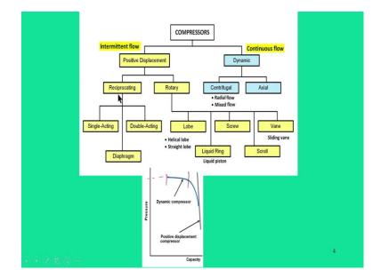
So, let me start with this compressor. Under the broad roof of compressors, there are many categories and we will be only focusing on reciprocating compressors. Now, if you look at the compressors, there are two broad categories, one is positive displacement type, other is dynamic type.
