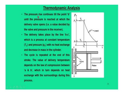
How long pressure keeps on rising? It goes rising till the point b until the pressure is reached at which the delivery valve opens. That means, till we reach this desired pressure  $p_2$ , the delivery valve opens, and its value is decided by the value and pressure in the receiver. So, delivery means it goes to another container or receiver where the needs to be stored.
