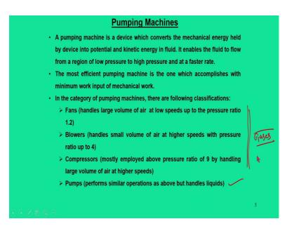
So, let me start this compressor with an introduction of what is a pumping machine. So, a pumping machine is a device which converts the mechanical energy held by the device into potential and kinetic energy of the fluid. Through this process it enables the fluid to flow from a region of low pressure to a high pressure and at a faster rate. The most efficient pumping machine is the one which accomplishes minimum work input for the mechanical work, for which it is intended.
