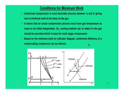
Now, what we can see is that if you try to recall this diagram in a TS plot and there are two pressure ratios  $p_1$ ,  $p_2$ , and isothermal process will take you in a straight line which is parallel to entropy axis.
