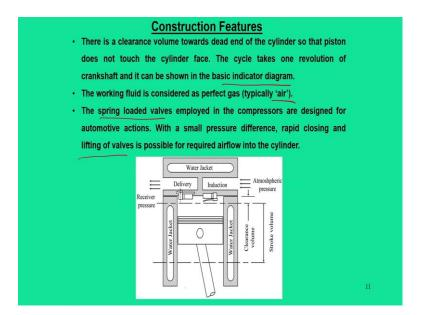
So, there is a clearance volume which I have already mentioned that towards the dead centre of the cylinder, so that piston does not touch the cylinder face. That is the first requirement. This cycle takes one revolution of the crankshaft and it can be shown as a indicator diagram. The word indicator diagram in thermodynamic sense we call this as a pressure volume diagram.
