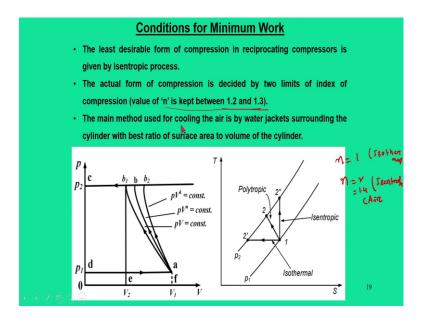
Another important point that I need to emphasize that what is the value of n typically maintained. So, as I mentioned the least desirable form of compressions in a reciprocating compressor is given by an isentropic process.
