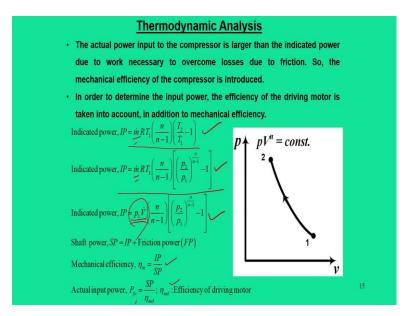
Now, moving further, now come up with expressions that indicated power which is  $\dot{m}RT_1\left(\frac{n}{n-1}\right)\left(\frac{T_2}{T_1}-1\right)$ . And putting this  $\frac{T_2}{T_1}$  as a function of  $\frac{p_2}{p_1}$ , because many a times pressures are measurable quantity. So, the working equation for a compressor now becomes is indicated power  $IP = \dot{m}RT_1\left(\frac{n}{n-1}\right)\left[\left(\frac{p_2}{p_1}\right)^{\frac{n-1}{n}}-1\right]$ .
