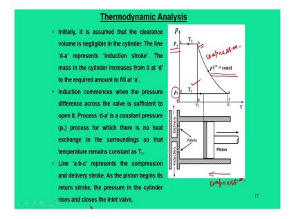
Now, let us see the thermodynamic nature or analysis for this reciprocating action of a gas in a compressors. And this schematic representations shows that the location of piston in any arbitrary positions.
