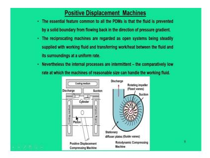
The other important essential features of positive displacement machine is that, fluid is prevented by the solid boundary from flowing back in the direction of pressure gradient. The reciprocating machines are regarded as the open systems being steadily supplied with working fluid and transferring work or heat between the fluid and its surroundings at uniform rate.
