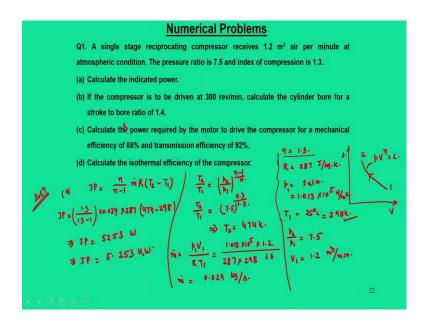
Now, we will try to solve a numerical problems based on the discussions what we have learned today. So, the question that was given that we have a single stage reciprocating compressors. It receives  $1.2 \text{ m}^3$  of air per minute at atmospheric conditions. That means, atmospheric air enters to the compressors at a flow rate of  $1.2 \text{ m}^3$ .
