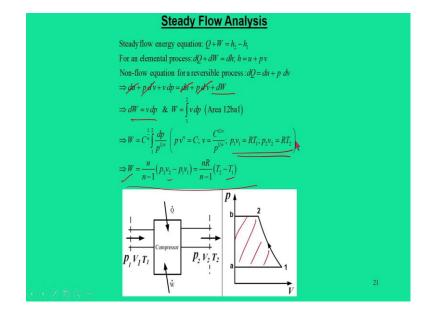
So, if you can recall our steady flow energy equation again from the first law for open system by neglecting kinetic energy and potential energy, we can write  $Q + W = h_2 - h_1$ and here for an element process dQ + dW = dh.
