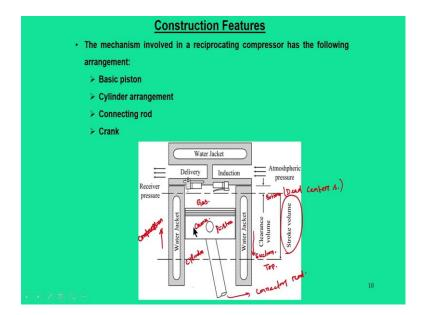
Now, let me come to the construction features of a reciprocating compressors. So, looking at the figure what we have seen is that we have a cylinder, which is housing a piston. So, we can call this as a piston, and we have cylinder and this piston is connected to a connecting rod, separately.
