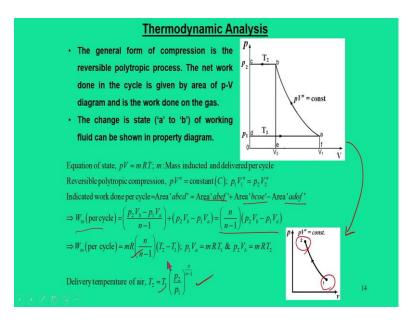
Now, from these we can frame a general thermodynamic equations how much mass gets inducted, and how what is this thermodynamic processes and how much work is required to compress certain slog of mass.
