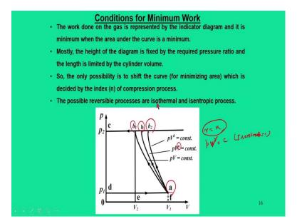
Another important segment of this compression work is that conditions for minimum work. So, an ideal compressor is the one which consumes minimum work for a given pressure ratio. So, the work done on the gas is represented by the indicator diagram, and it is the minimum one, under the curve is minimum.
