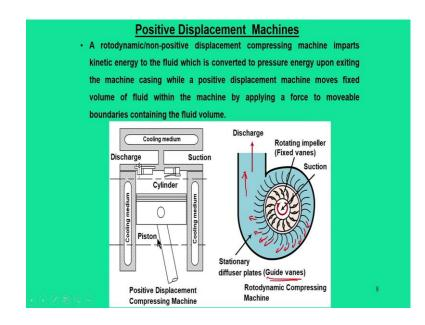
The, another way of classifying this pumping machine is a positive displacement and rotodynamics displacements. So, if you can the see this kind of a graphical or construction picture of a positive machines and a rotodynamic machines. What we can see? In a positive displacement machines, we have a piston cylinder, we have suction and we have discharge. So, we will discuss more details on this.
