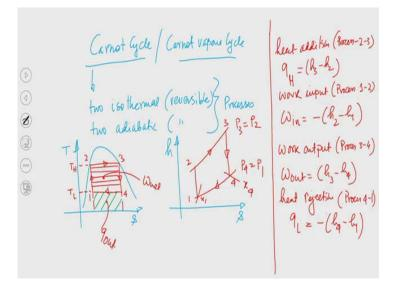
So, as I said this Carnot cycle to be precise Carnot vapour cycle. So, as I said that there are two efficiencies; one is ideal cycle efficiency, other is the actual cycle efficiency we have seen. But, again I am telling though it is difficult to achieve the ideal cycle efficiency in practice, but still we need to analyze it because we need to compare the
