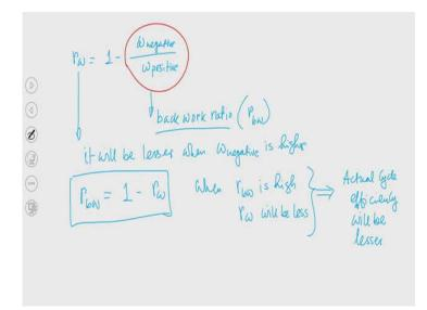
So, this work ratio  $r_w = 1 - \frac{w_{negative}}{w_{positive}}$ . So, this is the work ratio. You can understand that the ratio of negative work to the positive work is a decisive factor for the efficiency of the plant. So, we are supplying energy at the cost of this energy you are getting work output, but that work output but this is not the net work output. Though it is positive work, but this is not the net work.
