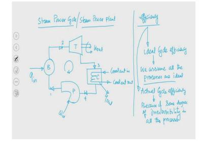
So, if we try to recall what are those equipment? So, if we write steam power cycle or I can write steam power plant briefly we will draw this line diagram which we have seen in the previous class. If we give the name this is 1, this is 2, this is 3 and this is 4, and this is the circuit or this plant is running in a cyclic manner.
