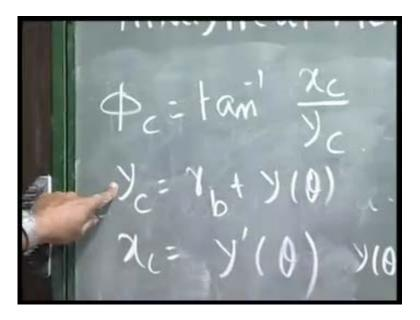
Phi<sub>C</sub> is tan inverse  $x_C$  by  $y_C$  and if we remember  $y_C$  is nothing but  $r_b$  plus y theta, and  $x_C$  is y prime theta. So given  $r_b$  and y theta, I get  $x_C$  and  $y_C$  so I get phi<sub>C</sub> and then I can get  $r_c$  and phi<sub>C</sub> prime and to get the polar coordinate representation of the cam profile with  $O_2$  as the origin. I will continue now this, for the similar exactly same technique for the roller follower.
