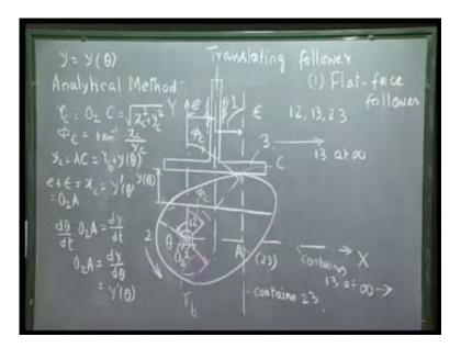
We know that how to size the cam that is, how to choose the value of the base circle radius and the proper amount of offset, the next task is to synthesize the cam profile to generate the desired follower motion given by y equal to y theta. We start with analytical procedure. For the time being, we are restricting our discussion to translating follower and first, we discuss if we have a flat face follower.
