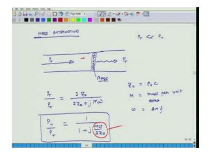
So, the first thing is mass attenuation. So, whenever I have some sound which is traveling across in a medium and I want to reduce the level of noise at the other end, then I can do it in 2-3 different ways. The first way is that I look up put a heavy piece of mass as an obstacle for this sound and then, less amount of sound gets transmitted across this
