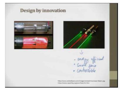
So, this is what the earlier laser design, we used to have a valve based system, today they have completely changed into the diode based system this is more energy efficient energy efficient and it occupies small space and it is controllable; that means, to say selectively tunable.
