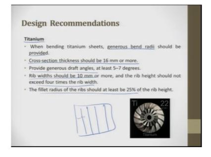
Titanium is one material which is talked about more in aerospace, biomaterial, and nowadays in automobiles. So, here when bend; when bending and titanium sheet generous bending radius should be provided, the cross section should be 16 millimetre or more, the cross section thickness, whatever it is a because when you try to machine titanium the heat gets accumulated at the cutting zone.
