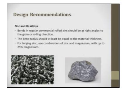
Zinc and its alloy. So, zinc is also nowadays becoming little general to use for various applications. Bending is regular commercial rolled zinc should be at right angles to avoid green or directional green or rolling directions. The bend radius should be at least equal to the material thickness. The forging zinc used a combination of zinc and manganese which put up to 25 percent. So, these are some of the nipples which are made out of zinc for various applications uses zinc alloyed.
