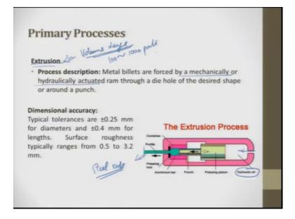
Next one is a metal forming process. So, this process is nothing, but an extrusion. So, extrusion what we do is we try to keep we try to keep the raw material. Raw material inside a die and then here you see there is a punch which is pushing and this punch is activated by the hydraulic system, whatever is there and this tries to give you the pressure.
