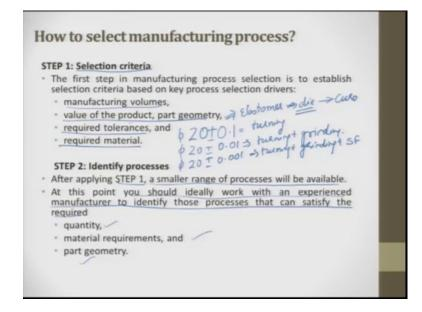
So, the selection the first step is selection criteria as have to be returned; manufacturing volume. In manufacturing, there is nothing called a unique solution. Suppose, if I want to produce a shaft of 10 numbers, then I use machining process if I have to produce something like 100 or 1,000 I always go for a rolling process. So, you see depending upon the number, depending upon the cost which you can pay for the product the process differs.
