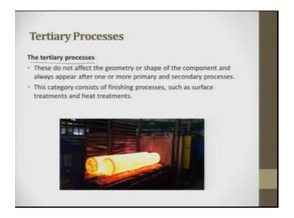
The last operation is heat treatment. So, heat treatment, as you have made a shape, you have made a size, but you wanted to play with a mechanical property alone. So, what we do is, we try to heat the work piece and then, after heating the work piece, we try to leave it in the atmosphere; furnace atmosphere or we try to bring it out and then, we try to go quenching. So, here what happens, only the mechanical properties keep changing.
