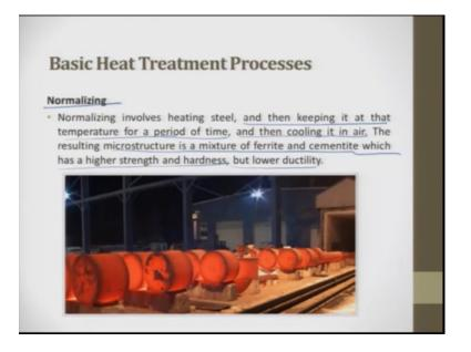
Normalizing involves a heat treatment. Here, heating steel here I have taken only an example of steel, you can also try to do with copper, aluminum, anything. Ok? For everything, there is a heat treatment cycle, you have to watch out for it and then, start doing it. I am walking through only steal, because steel is predominantly used material for primary structure load bearing area.
