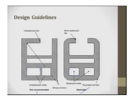
So, this is called as an unbalanced die. So, this is called as a balanced die. This is desirable, this is not desirable sharp edges are never desirable in punching operation, it is always good to have a fillet at radius, because sharp, when it is piercing, making a die is also a challenge because if it has to be punched. So, to have a punch which is square, making a square geometry is little difficult. So, if you have to, if you can make a filtered one. So, the sharp edges can be avoided.
