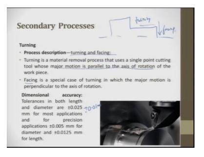
So, turning and facing have taken little bit. Turning is a material removal process where in which; we use a single point cutting tool. So, it moves whose major motion is parallel to the axis of rotation, of the work piece and facing, So, if I wanted to reduce a diameter. So, reduce a diameter. So, here this is, this is along the space parallel to the axis. The tool moves parallel to the axis. So, this is called Turning. If I move perpendicular to the axis, then it is called as Facing.
