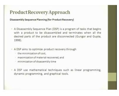
That they will say that after 10 years if you come back to me, I will try to put a better value for the product, and then I will try to give a discount for the product what you are giving it back to me; So, the disassembly sequential plan for product recovery. The disassembly sequential plan which is otherwise called as DSP, is a program of task that begins with the product to be disassembled and terminates when all the desired parts of the product are disconnected.
