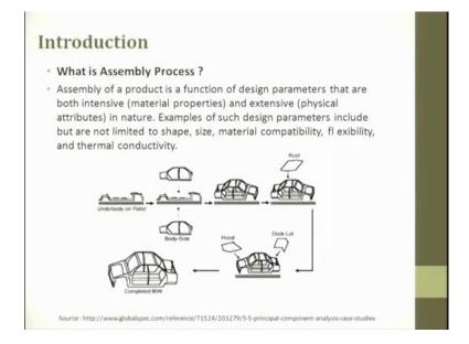
What is assembly it is a process, where in which we try to join or we try to consolidate number of parts and make a single product or make a part of a single product; such that it can meet out to some requirements. So, assembly of a product is a function of design parameters that are both intensive and extensive. Intensive is material property, extensive is physical attributes.
