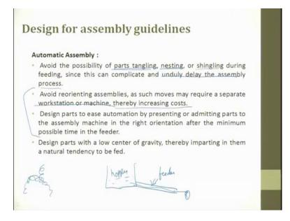
The automatic assembly guidelines, avoid the possibility of part tangling, nesting and shingling during the feeding. So, when you say automatic, automatic you will always have a hopper, then you will have a feeder. So, this is hopper, wherein which you put all
