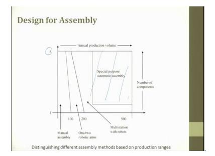
When we talk for design for assembly, here we have said 1 to 5 and then here are these numbers are given. Please these numbers are not sanctity numbers, these numbers are just taken for representation. So, here in this graph we clearly distinguish between assembly methods based on the production range. So, if you want to do manual assembly, you can the number of parts which you produces very less or the variety is very less and the production rate is also somewhere close to 100.
