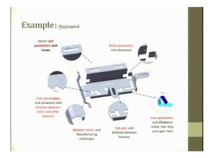
Sheet metal example; so, detects slot parameters and issues. So, here this is a slot which
