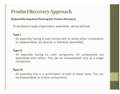
So, the disassembly sequence plan for product recovery has three distinct type of geometric assembly can be defined; Type 1, type 2, type 3. Type 1; an assembly having a main component to which other components or disassemblies are directly or indirectly assembled; for example, breadboard, PCB. Type 2, an assembly having low main components or components are assembled with each other, this may can be disassembled only as a single component.
