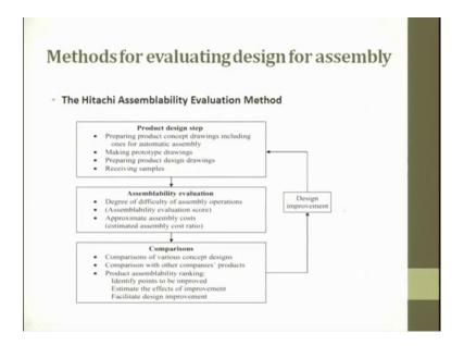
So, the Hitachi Assimilability Evaluation Method goes like this, product design step, prepare product concept drawing including ones for automatic assembly, making prototype drawings, preparing product design drawings, receiving samples. Then assimilability evaluation, degree of difficulty of assembling operation and then approximate assembling costs. So, these two comes here.
