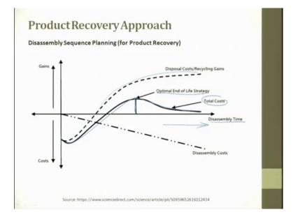
Disassemble sequence planning for product recovery, if you see gain and costs and then if you see here, this is the disassembly time we do. So, if you try to take this disposal costs and recycling costs, it gains over a period of time, disassembly time.
