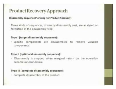
So, the three kinds of sequences driven by disassembly cost are analysed on formation of disassembly tree. So, here type one is target disassembly sequence, the special components are disassembled to remove valuable components. Type 2 is optimal disassembly sequence, disassembly stops when marginal return on the operation becomes uneconomical. Complete disassembly sequences, complete disassembly of the product.
