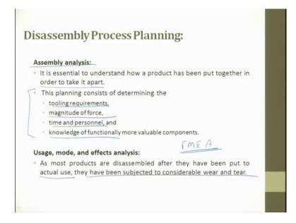
Assembly analysis, it is essential to understand how a product has been put together in order to make it a part. This planning consists of tool requirement, magnitude of force, time and personnel and knowledge of the functional, more valuable components. So, these are important things which we have to plan.
