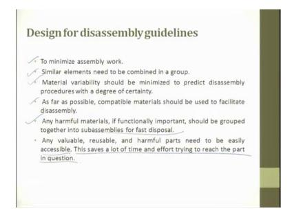
Since, only the intensive property of the components are important, destructive disassembly can be used to quicker the process. So, the design for disassembly guidelines, to minimise the assembly work, similar elements need to be combined together, it is just a repeat, material variability should be minimised. So, as far as possible compatible material should be used, any harmful material, if functional important should be grouped together into subassembly for fast disposal.
