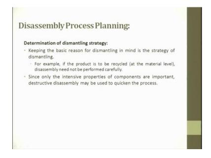
And decide for process analysis; Disassembly process planning, determination of dismantling strategy. So, we have seen the first three points here; product analysis, assembly analysis, usage analysis and then we are trying to see the determination of dismantling strategy. So, keeping the basic reason for dismantling in mind, the strategy for dismantling is. For example, if a product is to be recycle at the material level, disassembly need not be performed carefully.
