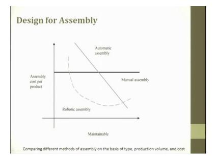
So, when you try to plot assembly cost per product was is maintainability. So, you can see there this is manual assembly, which is a straight line, the automatic assembly, the assembly cost per product, initially will be very high and slowly after a period of time it
