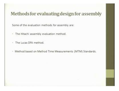
Some of the methods for evaluating design for assembly. So, one is Hitachi assembly evaluation, next is Lucas DFA method, the third one is Methods Time Measurement Standards.
