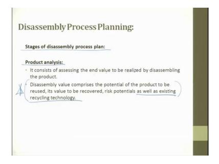
The stages of dismantling process plan, you have product analysis, functional analysis product analysis, it consists of assessing the end value to be realised by disassembling the product ok, it consists of assessing the end value to be realised by disassembling the product.
