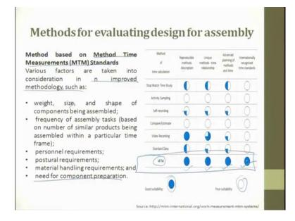
In method based on method time measurement standards, various factors are taken into consideration in n improvement methodologies; such as weight, size, shape of the component being assembled; Frequency of assembly task, personal requirements, postural requirements, sitting down.
