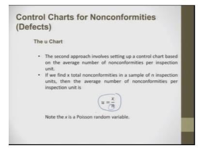
So, it is used by a chart called as u chart. So, the u chart is nothing, but x / n where, x is the total nonconformity in a sample and n is the inspection in a sample of n inspection. So n unit inspection, this is n is number of samples along and x is the total nonconformity in a sample.
