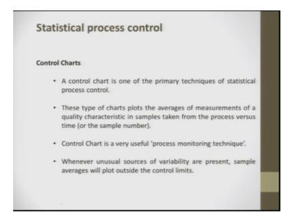
A control chart is one of the the primary technique of statistical process control. This type of chart plots the average of measurements of quality characteristics in samples taken from the process versus time ok. So, we try to take a product we try to take a part which is produced and this part can be ones in 50 parts or it can be ones in half an hour. So, we pull out and then try to check the various dimensions and deviations and note it down.
