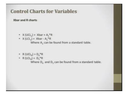
So, here are some of the formulas which are given. So, we are trying to figure out the upper critical and the lower critical value for X bar, upper critical and lower critical for R so all those things. You can expect the problem by I can give you a set of data then ask you to draw a control chart or ask you to find out some value from the control chart or ask you to try to figure out what is the lower critical limit, upper critical limit etcetera, etcetera.
