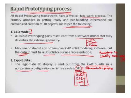
And next is the general process for Rapid Prototyping. So, all Rapid Prototyping frameworks have a typical data work process. The primary arranges in getting ready and pre-handling information for mechanized creation of 3D objects as per the following steps. So, first is having a CAD model.
