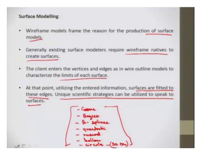
So, next is Surface Modeling, wireframe models frame the reason for the production of surface models, because in wireframe models these wireframes are there, but we do not have information in between what is there in this surface so, surface models were required.
