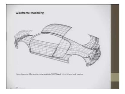
So, this looks like surface of the or the outer body of the car is made up of wires. So, these models these days we can use is when you use any software like solid works Katya NX or any like surface modeling software also so, these wireframe models are made by itself.
