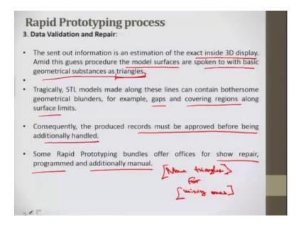
So, next step is data validation and repair, the sent out information is an estimation of the exact inside 3D display, that is we need to produce. Amid this guess procedure of the model surfaces are spoken to with basic geometrical substances as triangles. So, these all data points are brought to be made up of triangles here.
