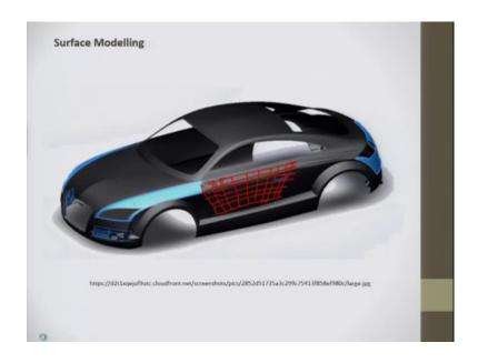
This is an example of a surface model of a car. So, the wireframe model is then the surfaces are filled this was a wireframe model. So, these surfaces are filled so, each of the element here is filled here.
