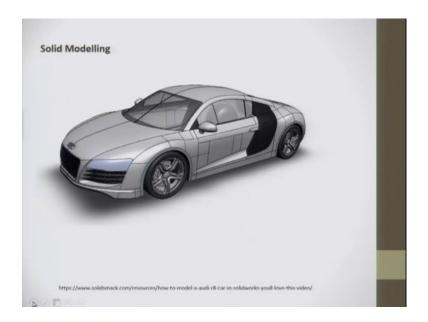
So, if I talk about this car, could this body outer body be made in one go? A could a single print made this? If I say yes it can be done by certain process lies the laser sintering process might do this thing. But if I talk about the wheels, these are different components, this is a different component and these different parts can be made separately and then assembled. If you just need to have the surface look, the shape look, the shape feel, then this can be manufactured in a single go.
