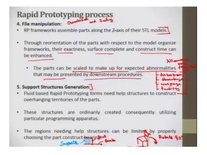
Then is file manipulation, here manipulation means orientation and scaling now, Rapid Prototyping frameworks assembles part along the Z axis of their STL model and sometimes to produce the parts, to manufacture the parts the orientation has to be made different. So, as them to say we have to see what is the support that is required, what are the hollow surfaces and what are the positive and negative surfaces.
