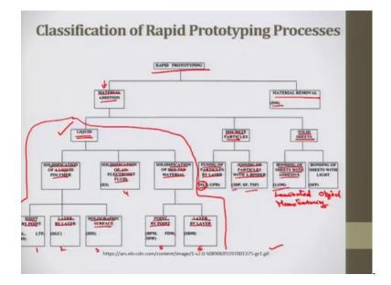
So, I will start with my classification thing, rapid prototyping can be classified into 2 ways first material addition and material removal. Actually these 3 are the materials, I would have to mention liquid, solid and discrete particles are the kinds of materials. So, here liquid discrete particles and solid sheets these 3 kinds of materials are used and we can see the most of the processes which are there use liquid material.
