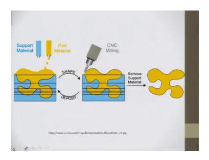
In this case what happens? The support material is provided here and layer by layer the part material and support material is there and support material is then removed using CNC milling that this figure very well explains how does this thing happens. So, in this case this shape deposition is there, the shape and deposit is being done alternatively.
