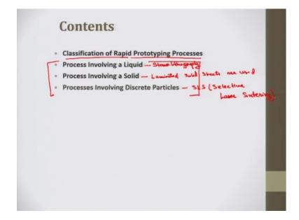
First, I will talk about the classification of rapid prototyping processes then we will discuss various kinds of prototype processes involving a liquid, processes involving a solid and processes involving discrete particles. In liquid the major or the common
