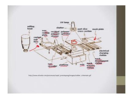
So, in this case specifically what we have a UV lamp and this is a mask, the UV light is passing through this mask and the only this portion from which light could pass through this portion would solidify this only this portion would be cured and other portion would not. Then the part slice cross section it is done another mask is put in for these successive layers.
