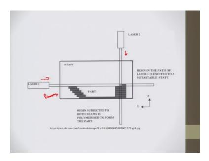
So, this is the kind of our beam interference solidification 2 lasers are at right angles, one is the primary laser another one is the secondary laser.
