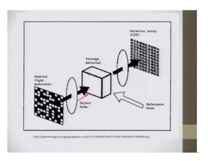
So, this is a specific kind of holographic interference solidification method. The spatial light modulator is there and the light is passed this is the storage material object beam is there, a reference beam is there and detector array is there.
