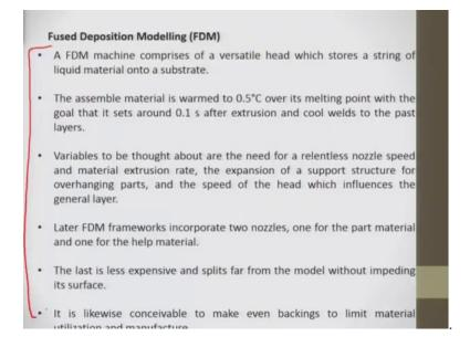
A next is Fused Deposition Modelling, this one also comprises of a versatile head which stores a string of liquid material onto substrate. So, please go through this as well.
