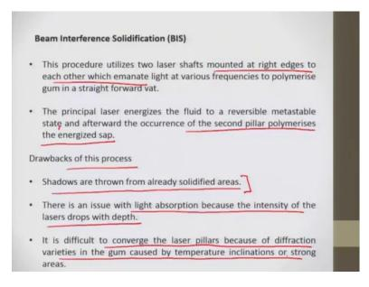
Now, next is Beam Interference Solidifications, this procedure utilizes 2 laser shafts mounted at right edges to each other which emanate light at various frequencies to polymerize gum in a straight forward to vat. The principal laser energizes the fluid to a reversible metastable state and afterward the occurrence of the second pillar polymerizes energized resin here.
