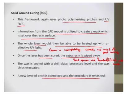
Now, next is Solid Ground Curing, this framework again uses photo polymerizing pitches and ultraviolet light. The information from the CAD model is utilized to create a mask which is set over the resin surface here. So, the whole layer would then be able to be heated up with an effective UV light, once the layer has been cured the extra resin is wiped away. Now, because the whole layer be heated up with the ultraviolet light this
