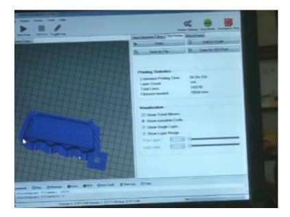
So, this brim is you can see. This cure is here. Why this cure is here? This cure is for holding. We need to hold the job and take it off. It holds the brim; hold the brim layer and take it off ok. This scale is for the holding and the other portion this outer portion is the brim because it has to it would like to save the edges or the make the edges proper brim is only at the edges it had been rough, it would be along all the surface complete surface of the job, ok.
